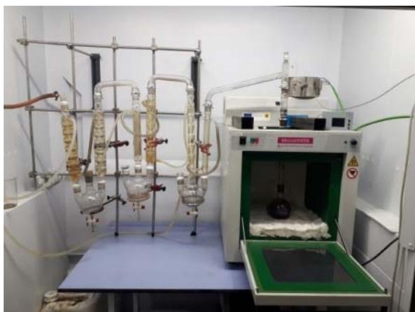
**Figure 1.** Pyrolysis prototype.
