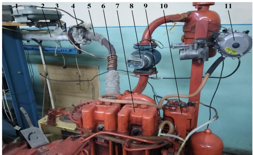
**Figure 3.** Appearance of the hydrogen supply system for the study of the experimental stand performance based on the diesel engine D21A1: 1—tank for liquefied methanol; 2—exhaust manifold of the engine; 3—filter; 4—gas collector; 5—thermal insulation of the exhaust manifold; 6—thermochemical reactor (thermal insulation is partially dismantled); 7—D21A1 diesel engine; 8—gas meter; 9—viewing window in the supply tube of gaseous methanol; 10—high-pressure diesel pump; 11—gas reducer.
