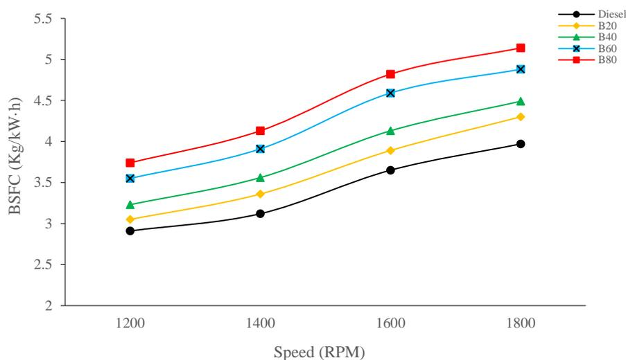
**Figure 9.** Variation of BSFC at different engine speeds and blends.
