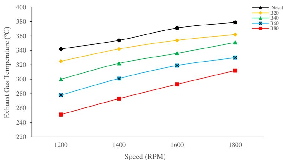
**Figure 10.** Variation of EGTs at different engine speeds and blends.
