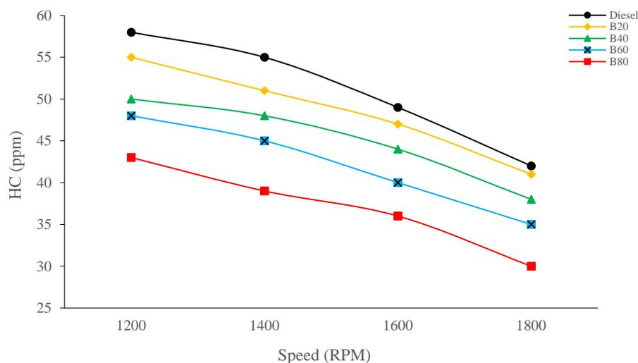
**Figure 5.** Variation of HCs at different engine speeds and blends.
