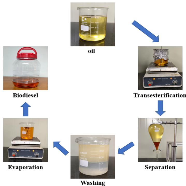
**Figure 1.** Castor biodiesel production process.
