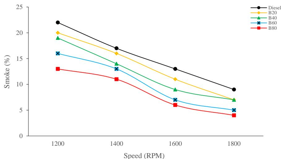
**Figure 7.** Variation of smoke at different engine speeds and blends.
