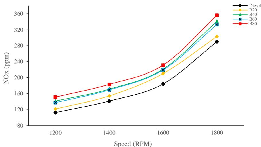
**Figure 6.** Variation of NOx at different engine speeds and blends.
