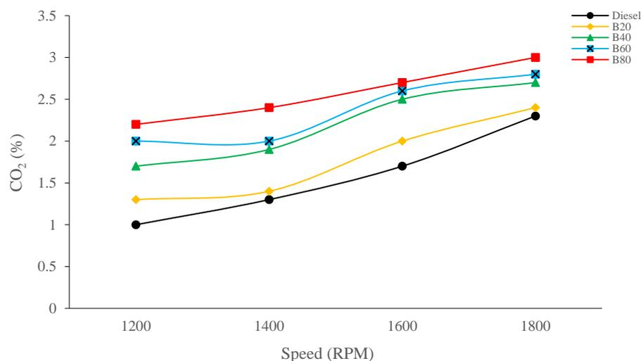
**Figure 4.** Variation of CO<sub>2</sub> at different engine speeds and blends.
