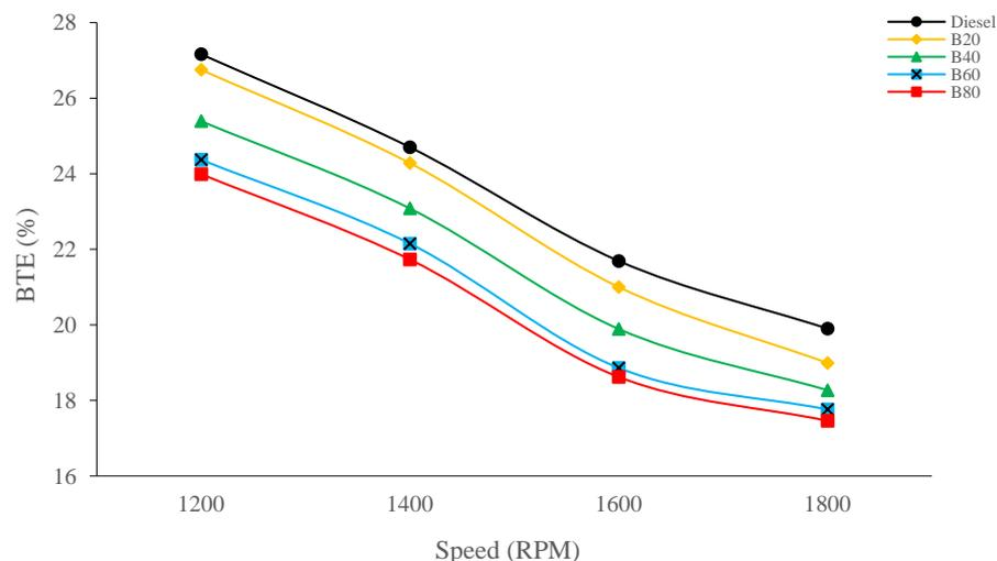
**Figure 8.** Variation of BTEs at different engine speeds and blends.
