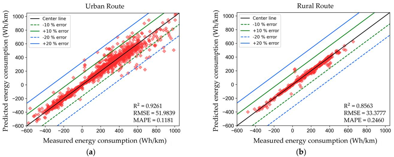
**Figure 3.** Plots of measured versus predicted values of the consumption of the BEVs under different route modes: (a) urban route; (b) rural route.
