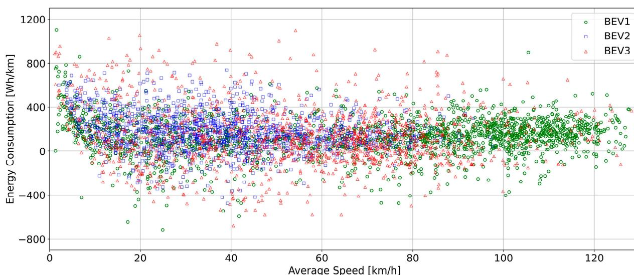
**Figure 2.** The energy consumption in relation to the average travel speed of the selected BEVs.
