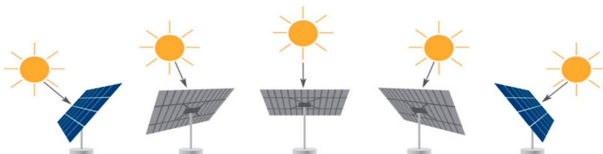
**Figure 7.** Orientation of photovoltaic panels towards the Sun (adapted from [42]).
