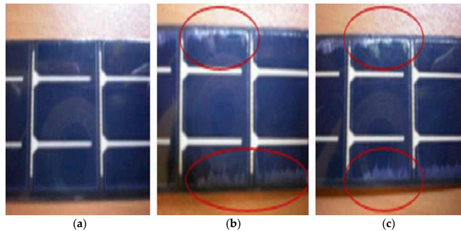
Figure 5. (a–c) Solar cells that received water (adapted from [38]).
