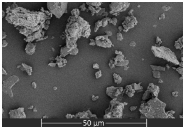
**Figure 4.** Structural SEM appearance of dust (adapted from [28]).
