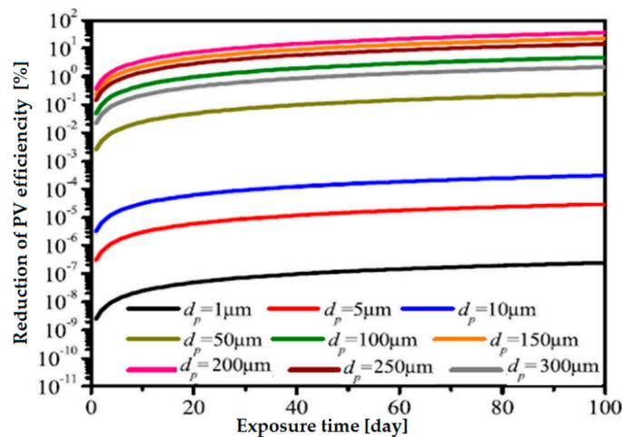
Figure 14. Effect of dust size on the efficiency of PV modules (adapted from [95]).
