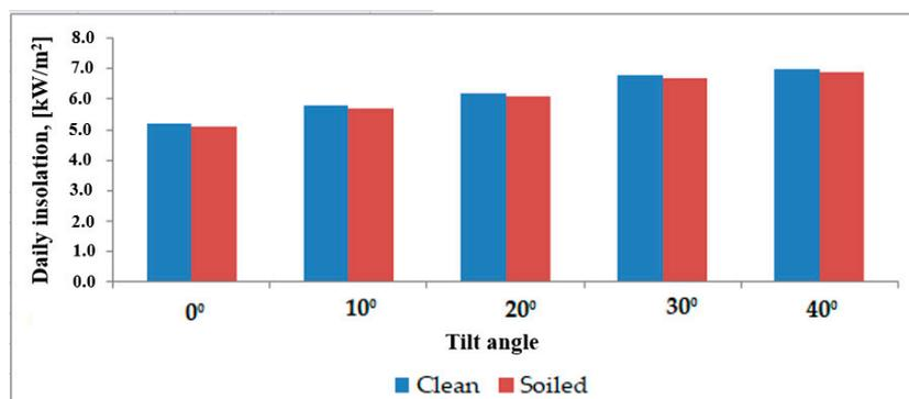
**Figure 8.** Average daily insolation values for dust-covered and clean PV panels as a function of tilt angles (adapted from [45]).
