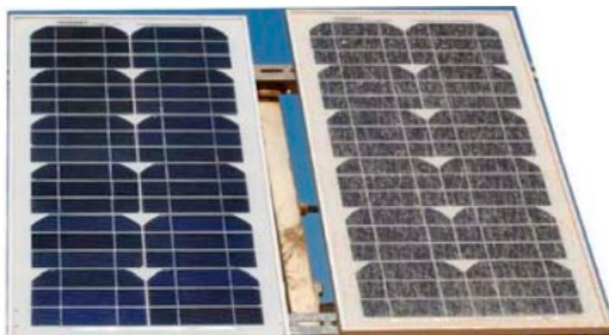
**Figure 3.** Solar panels covered in dust (adapted from [31]).
