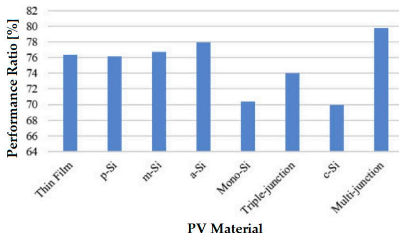
Figure 15. Performance ratio of photovoltaic panels (adapted from [99]).
