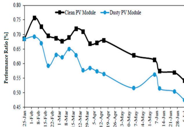
Figure 13. The ratio performance of clean and dust-covered photovoltaic panels (adapted from [95]).
