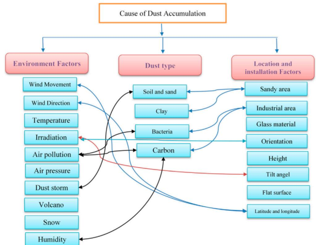
**Figure 1.** The causes of dust accumulation on the surface of solar panels (adapted from [24]).
