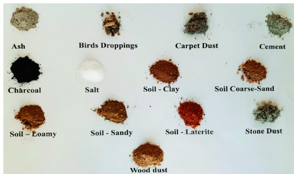
**Figure 2.** Dust samples that can be deposited on the surface of solar cells (adapted from [25]).
