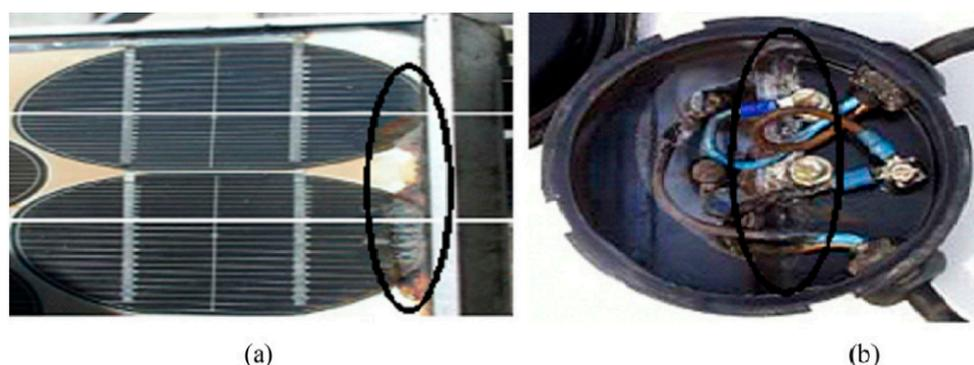
**Figure 9.** Corrosion effects on PV module at (a) edge and (b) junction box (adapted from [28]).
