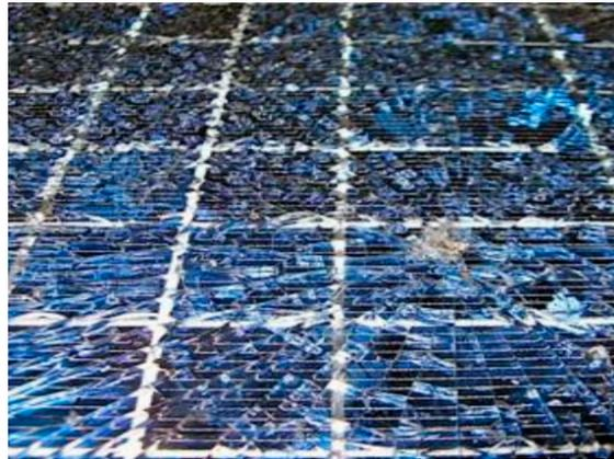
Figure 10. PV module with broken glass (adapted from [70]).
