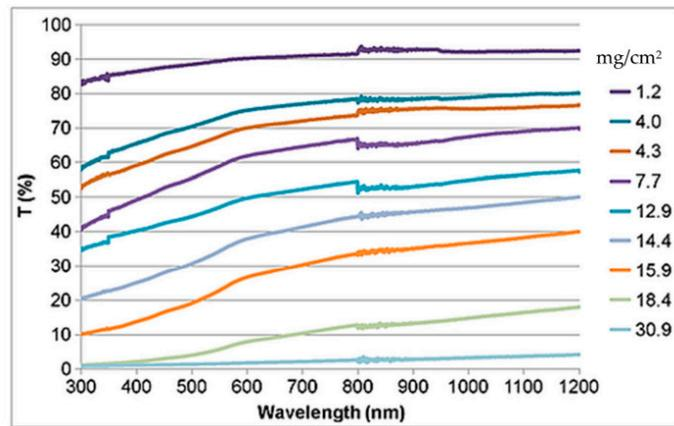
Figure 12. The variation of transmittance depending on the density of deposited dust (adapted from [5]).
