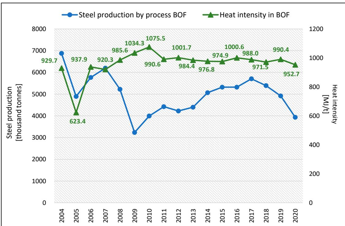
Figure 3. Heat intensity per 1 tonne of steel in the BOF process in Poland from 2004 to 2020. Source: Own elaboration based on data from [11].
