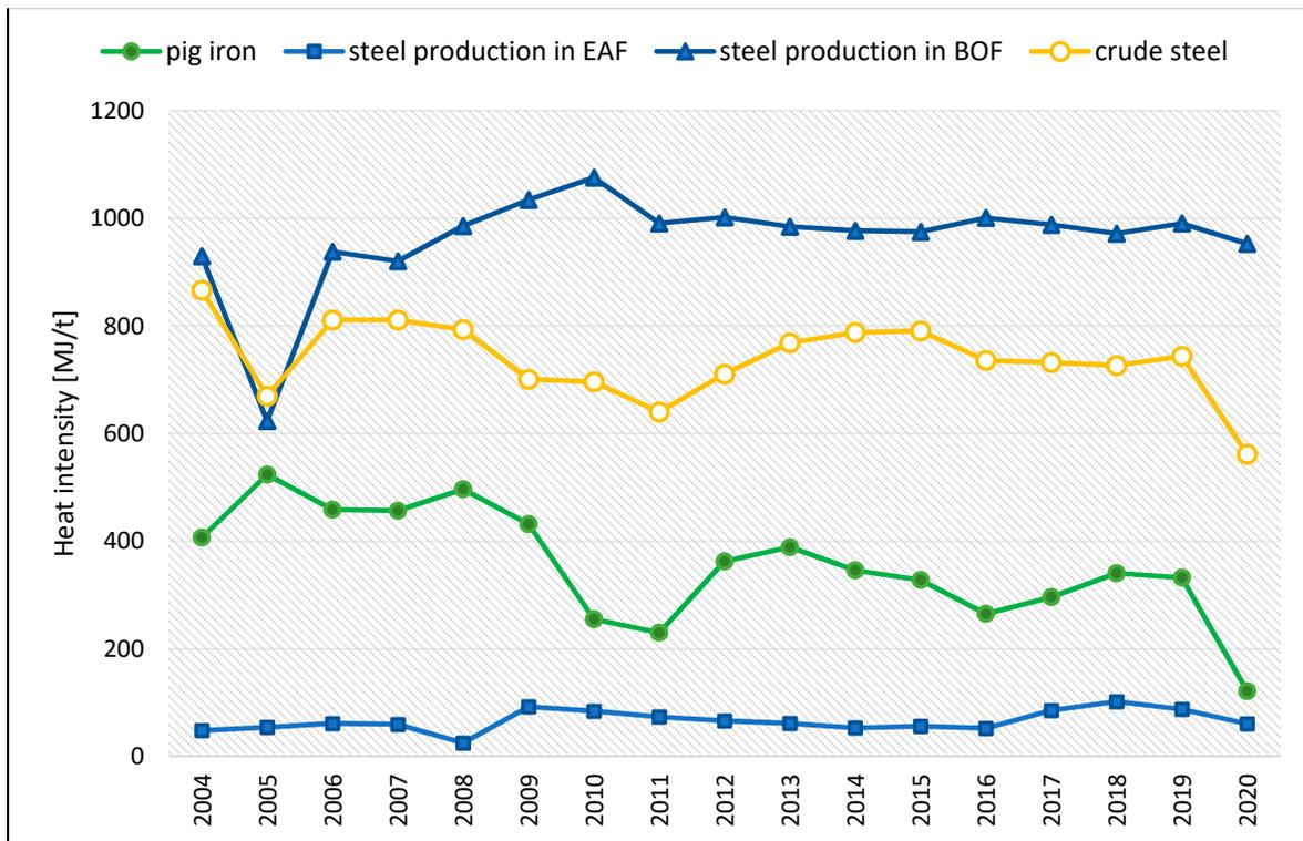
Figure 4. Heat intensity per 1 tonne of steel in all the metallurgical processes in Poland from 2004 to 2020. Source: Own elaboration.
