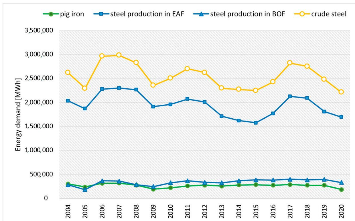
**Figure 13.** Total energy demand in all metallurgical processes in Poland from 2004 to 2020. Source: Own elaboration. Total energy intensity for the category: crude steel is the sum of energy intensity for production of pig iron with BOF and EAF.
