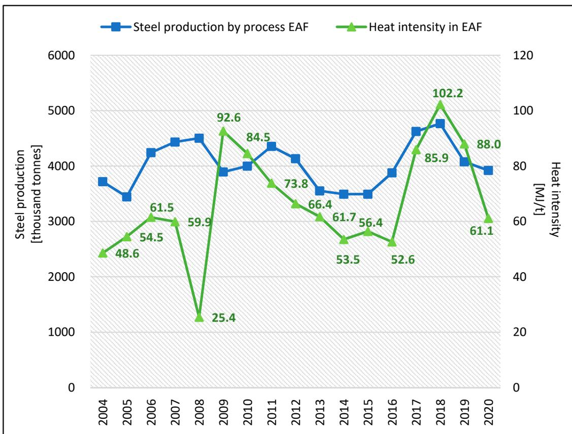
Figure 2. Heat intensity per 1 tonne of steel in the EAF process in Poland from 2004 to 2020. Source: Own elaboration based on data from [11].
