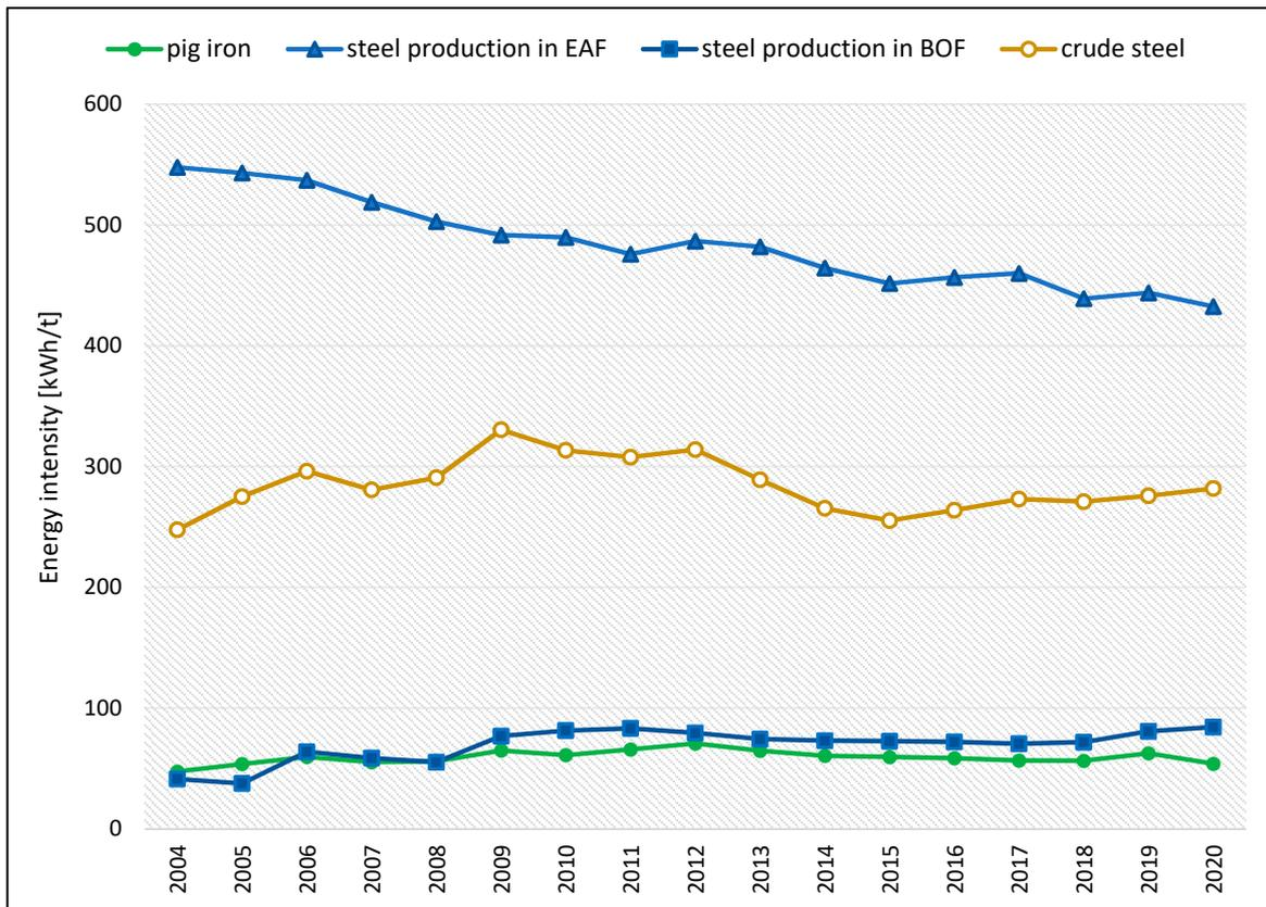
Figure 10. Energy intensity per 1 tonne of steel in Poland from 2004 to 2020. Source: Own elaboration.
