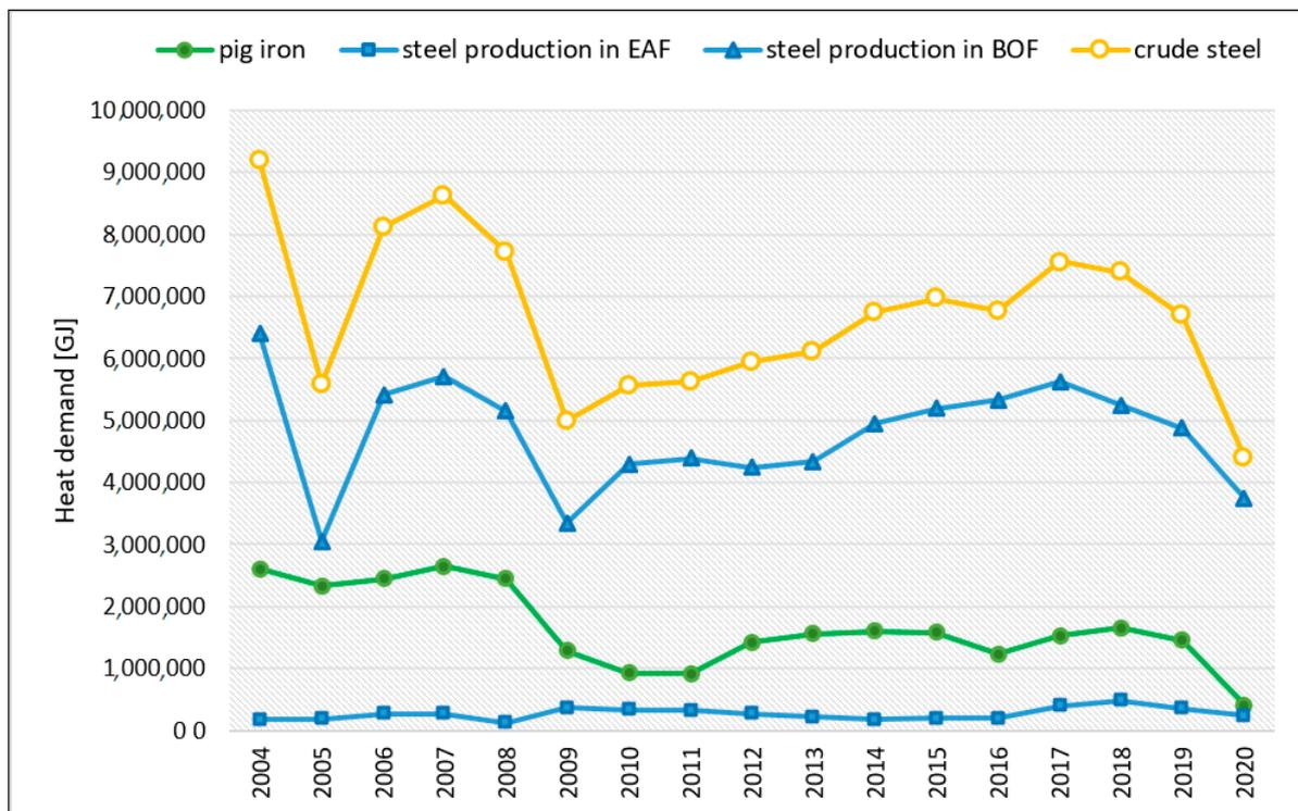
Figure 7. Total heat demand in all of the metallurgical processes in Poland from 2004 to 2020. Source: Own elaboration. Heat intensity for the category: crude steel is the sum of heat intensity for production of pig iron with BOF and EAF.
