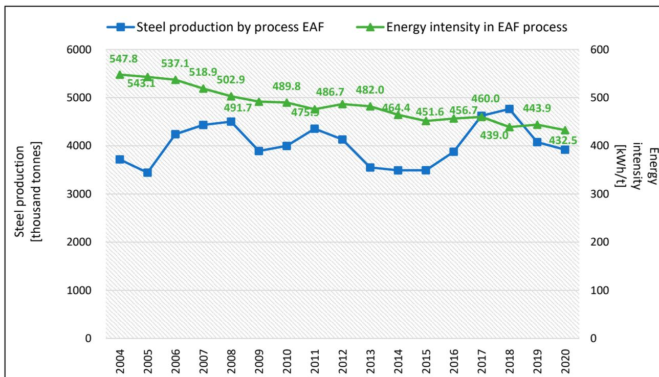
**Figure 8.** Energy intensity per 1 tonne of steel in the EAF process in Poland from 2004 to 2020. Source: Own elaboration based on data from [11].
