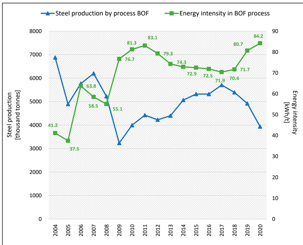
**Figure 9.** Energy intensity per 1 tonne of steel in the BOF process in Poland from 2004 to 2020. Source: Own elaboration based on data from [11].
