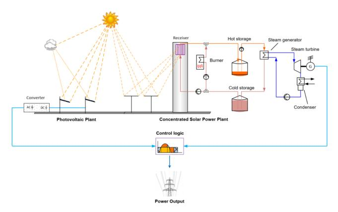
**Figure 5.** Sketch of a CSP + PV + gas burner hybrid plant (CP3 case).
