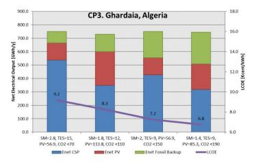
**Figure 7.** Energy production per configuration case (CP) and location. Solar multiple (SM), thermal storage capacity in full load hours (TES), nominal PV capacity in MW and  $CO_2$  emissions in g  $CO_2/kWhe$ .
