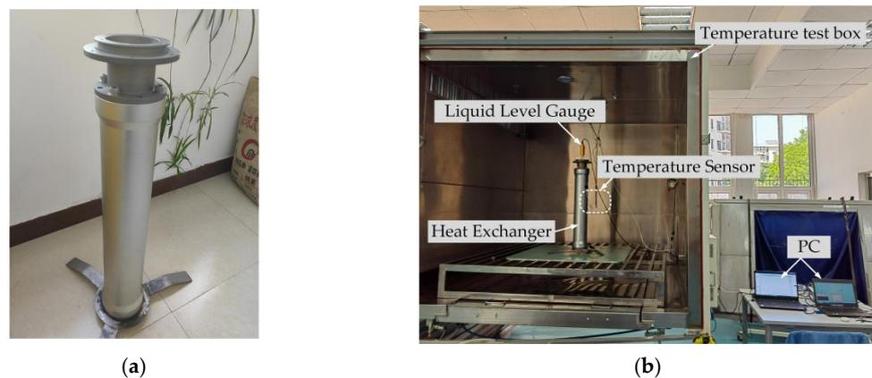
**Figure 7.** The heat exchanger prototype and the experimental equipment: (a) the heat exchanger prototype; (b) the experimental equipment.
