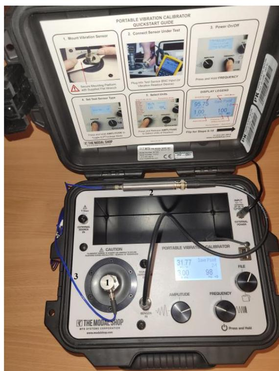
Figure 2. System for the standard calibration of the charge mode accelerometer using the portable calibrator of type 9110D. 1—accelerometer under test, 2—charge amplifier, 3—connection cable.
