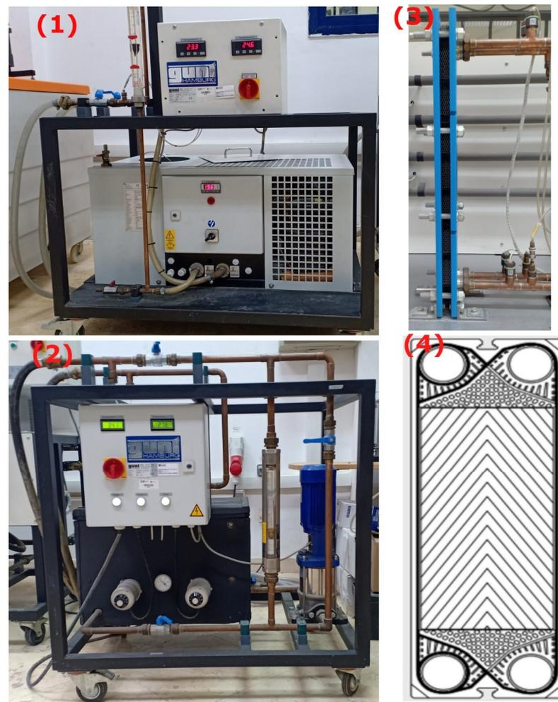
**Figure 2.** Experimental setup components consist of (1) CWB, (2) HWB, (3) C-PHE, and (4) corrugated plate channel of PHE.
