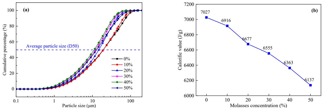
**Figure 1.** The particle size distributions (a) and the calorific values (b) of the explosion coal dust samples.
