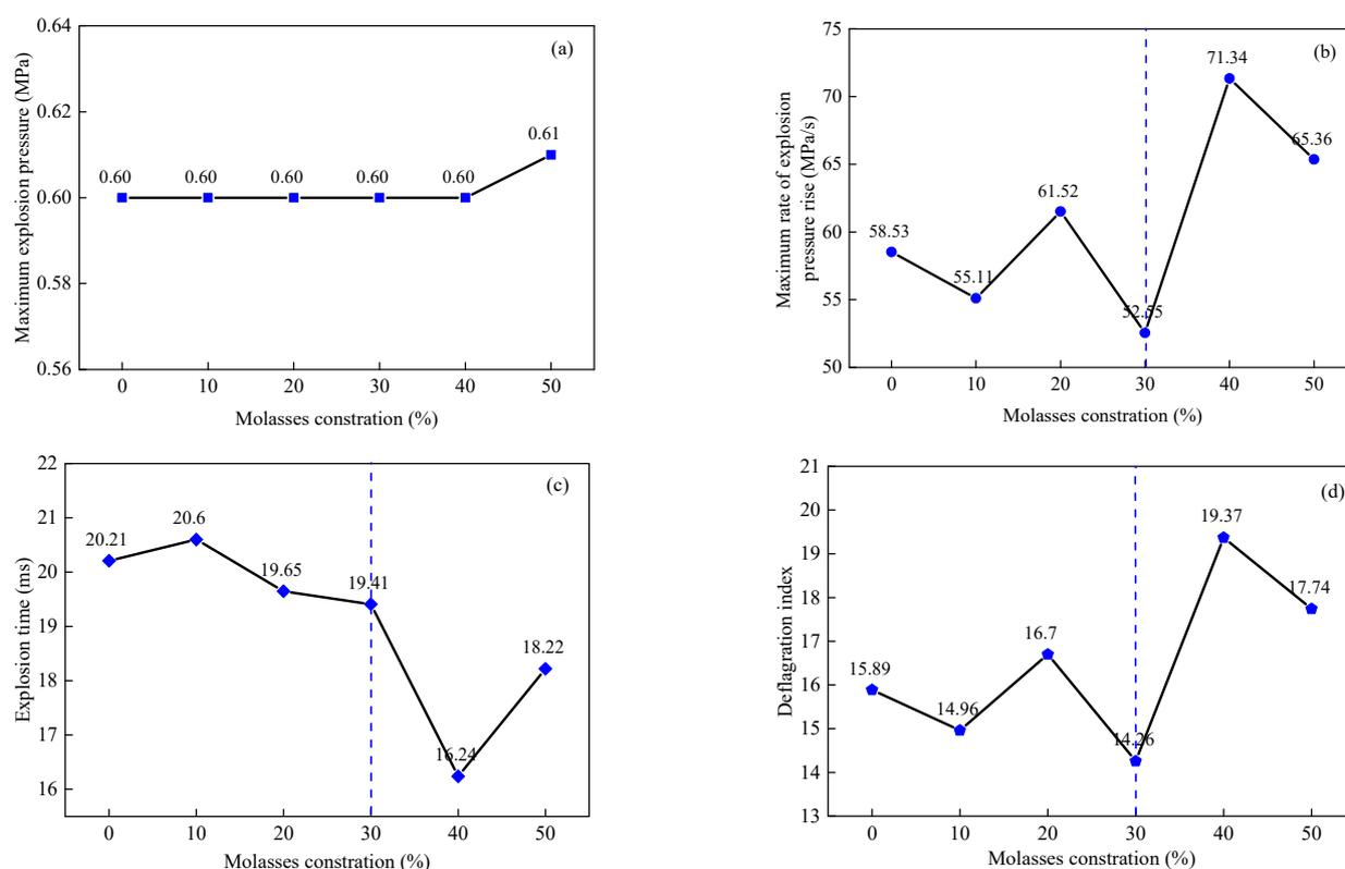
**Figure 7.** The maximum pressure (a), the maximum rate of the explosion pressure rise (b), the explosion time (c), and the deflagration index (d) of the explosion coal dust samples at a  $400 \text{ g/m}^3$  explosion concentration.
