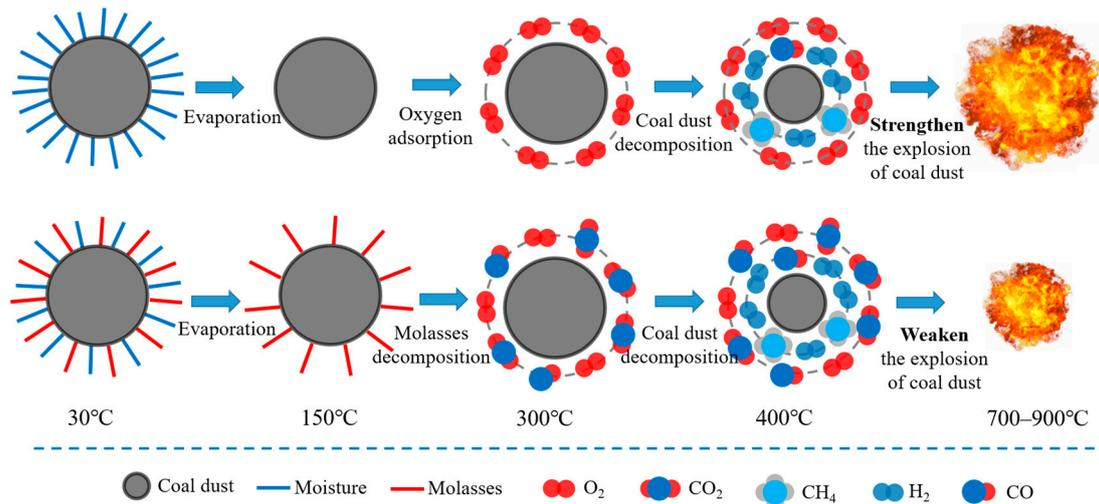
**Figure 12.** Schematic diagram of the influence of molasses on the coal dust explosion.
