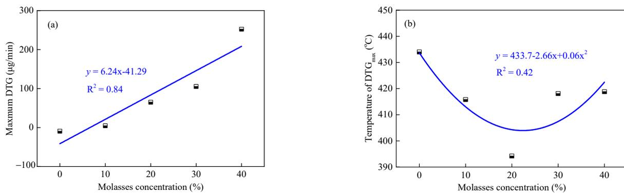
**Figure 10.** The maximum of the DTG ( $DTG_{max}$ ) at 150–300 °C (a) and the temperature corresponds to the  $DTG_{max}$  at >300 °C (b).
