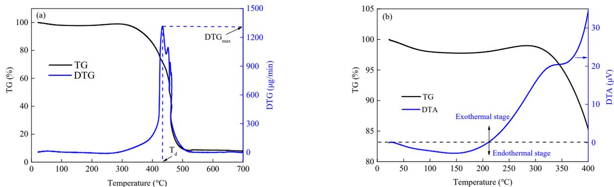
**Figure 4.** The typical thermogravimetric and derivative thermogravimetric (TG-DTG) curve (a) and the differential thermal value (DTA) curve (b) of the decomposition of coal dust.
