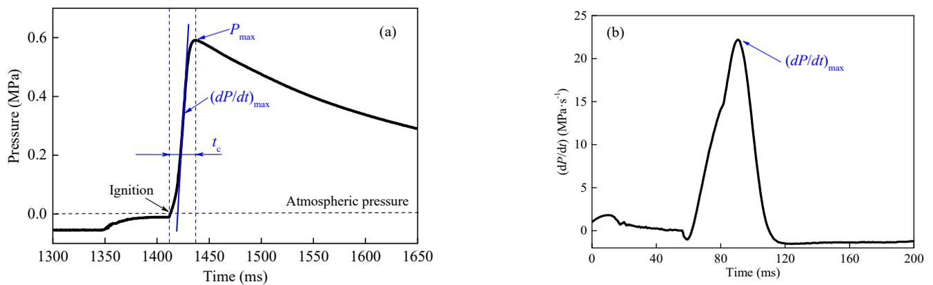
**Figure 3.** The explosion pressure (a) and the first-order derivative of the explosion pressure (b).
