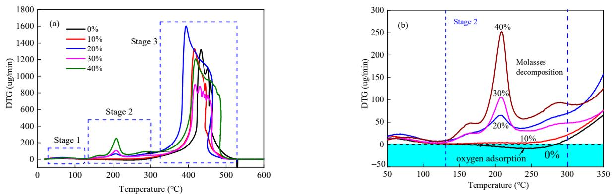
**Figure 9.** The DTG curve of the coal dust mixed with molasses at 0–600 °C (a) and 0–300 °C (b).
