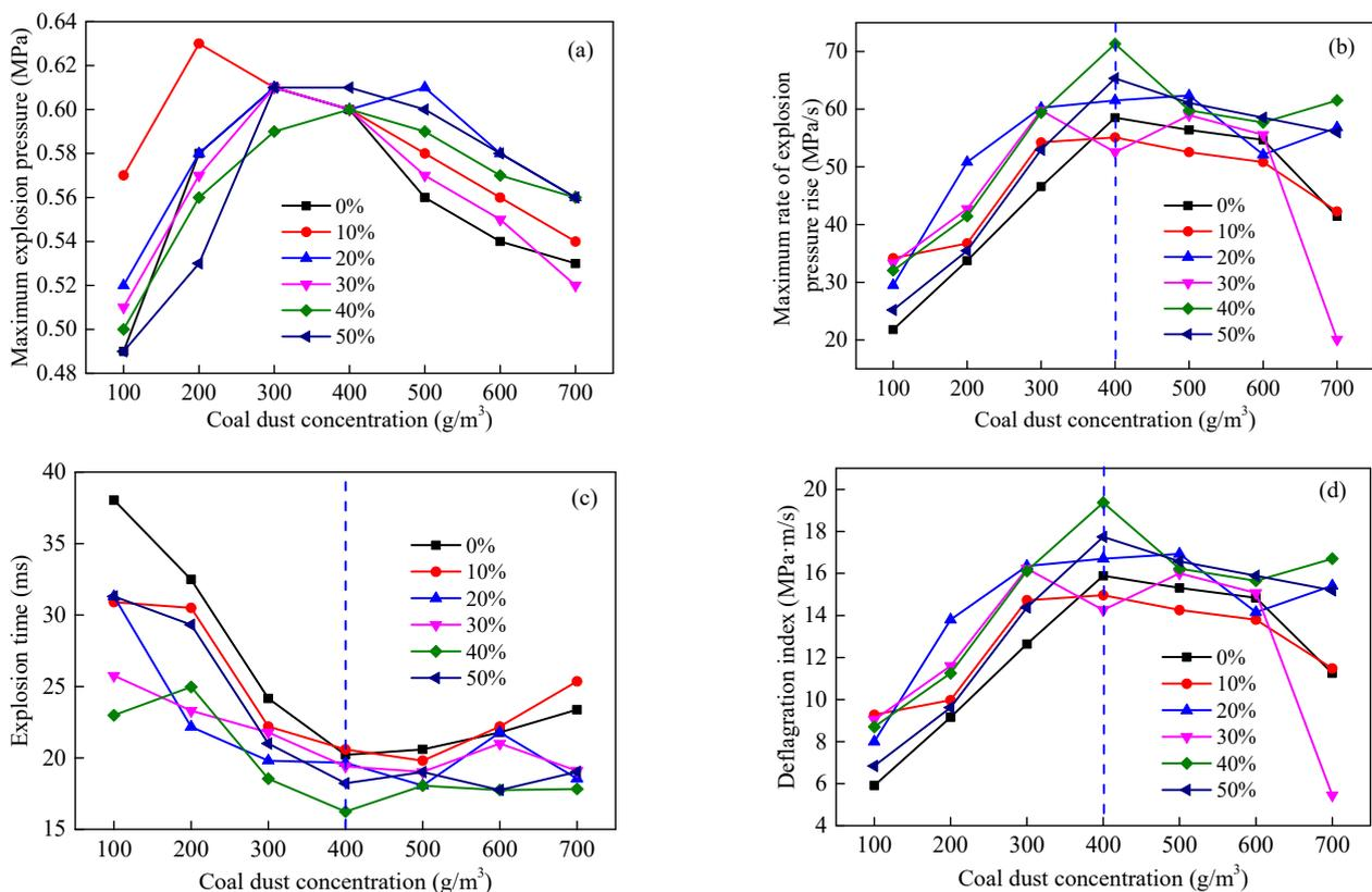
**Figure 6.** The maximum pressure (a), the maximum rate of the explosion pressure rise (b), the explosion time (c), and the deflagration index (d) of the explosion coal dust samples at a series of explosion concentrations.
