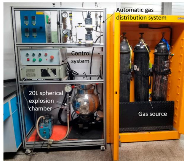
**Figure 2.** The 20 L spherical explosive device.
