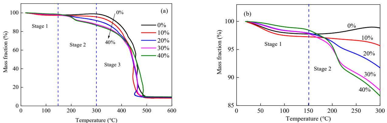
**Figure 8.** The mass fraction of the coal dust at 0–600 °C (a) and 0–300 °C (b).
