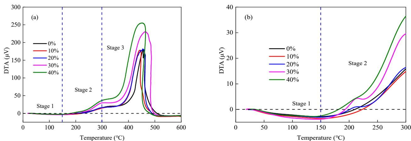
**Figure 11.** The DTA of the coal dust at 0–600  $^{\circ}$ C (a) and 0–350  $^{\circ}$ C (b).
