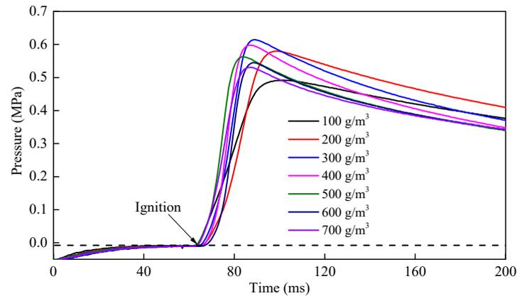
**Figure 5.** The explosion pressures of the coal dust mixed with a 0% molasses solution at various explosion concentrations.
