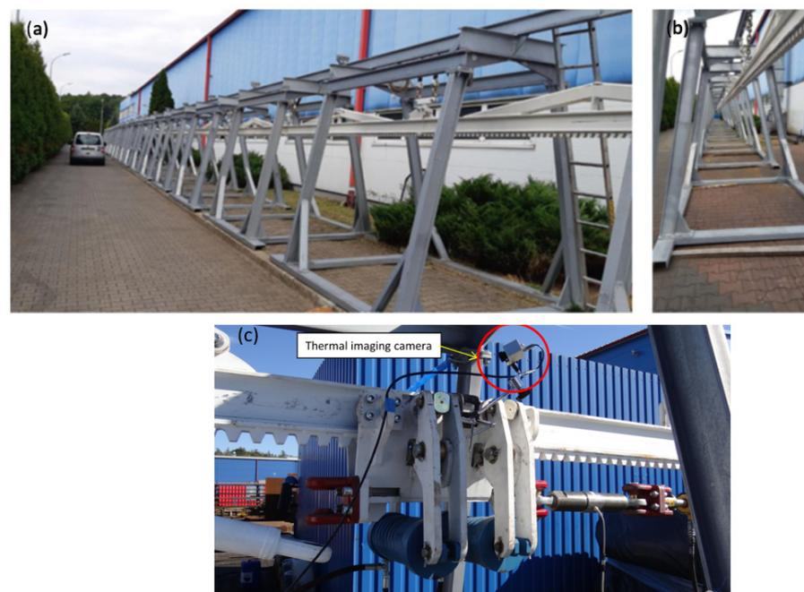
**Figure 2.** Overall view of the test track on the test stand (a); an operator's view (b); the way of mounting of the thermal camera (c) [25].
