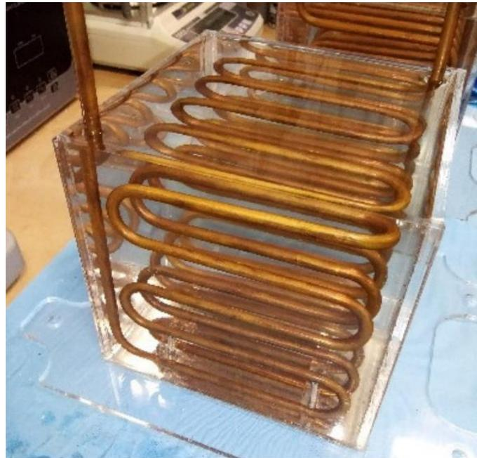
**Figure 4.** One of the three modules composing the PCM-based condenser without the thermal insulation.
