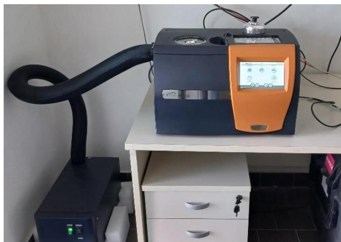
**Figure 1.** DSC 250 TA Instruments (Waters).
