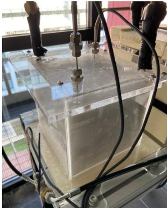
**Figure 19.** PCM-based condenser module in its initial condition.
