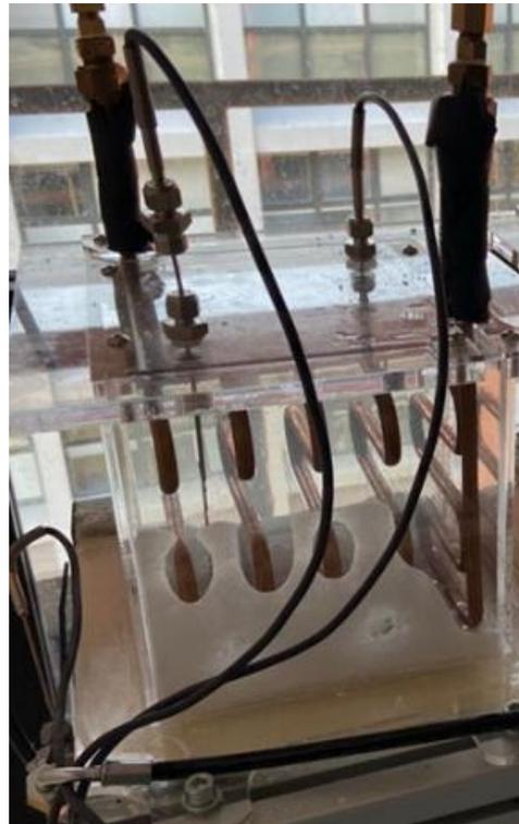
Figure 23. PCM-based condenser module after 3700 s.
