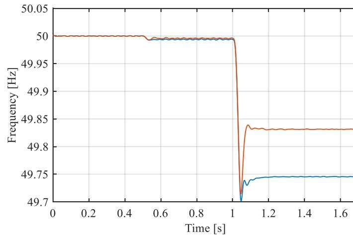
**Figure 8.** Frequency behavior during a load connection with (red line) or without (blue lines) PV system participating to PFR.
