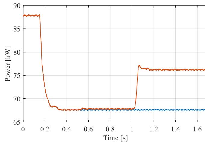
**Figure 9.** PV power injection during a load connection with (red line) or without (blue lines) PV system participating to PFR.
