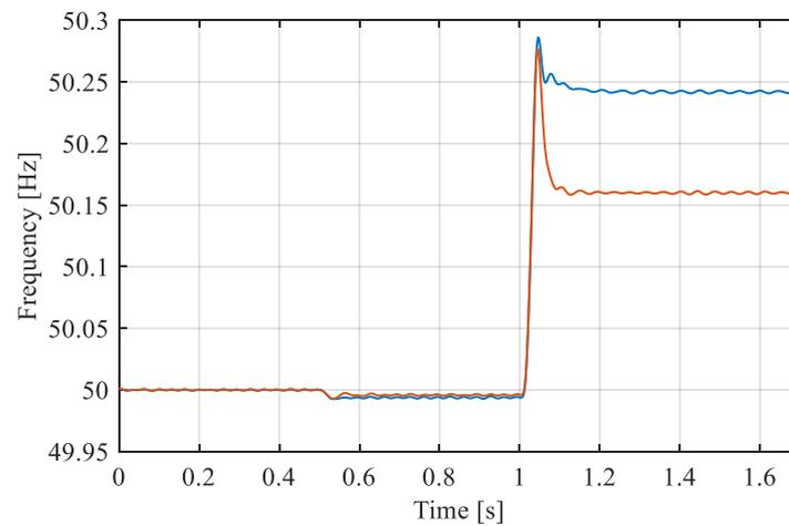
**Figure 10.** Frequency behavior during a load disconnection with (red line) or without (blue lines) the PV system participating in the PFR.
