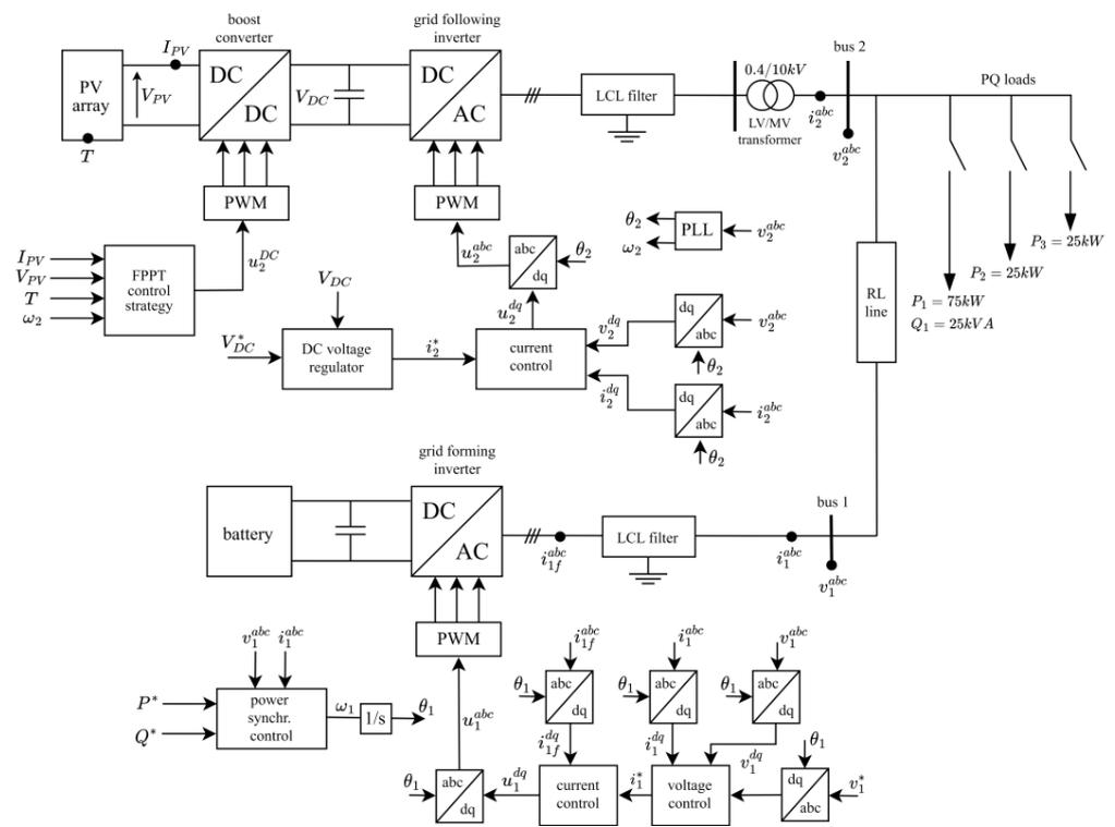
Figure 2. Grid-forming and grid-following inverters control.
