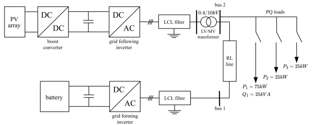
Figure 1. Simulated microgrid.
