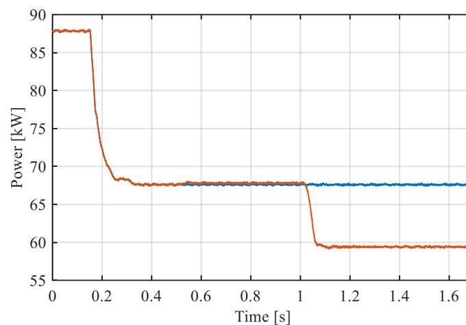
**Figure 11.** PV power injection during a load disconnection with (red line) or without (blue lines) the PV system participating in the PFR.
