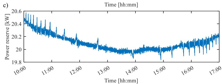
**Figure 6.** (a) Irradiation profile, (b) temperature profile (measured values in blue line and interpolated values in red line), (c) maintained active power reserve.
