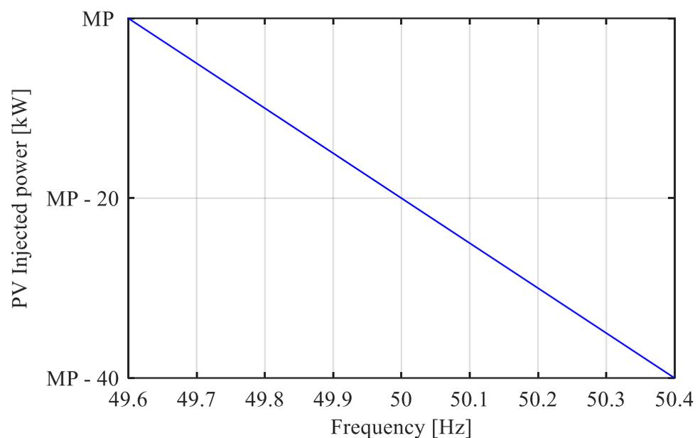
**Figure 7.** Implemented active power–frequency droop control.
