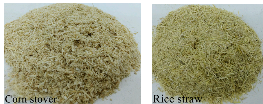
Figure 1. Raw material samples of corn stover and rice straw.
