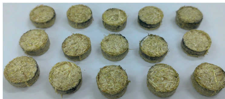
Figure 7. Pellets made from mixing material in confirmation experiments.
