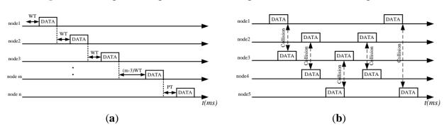
Figure 7. Timing of the algorithms. (a) Timing of the ACRA; (b) Timing of CSP.
