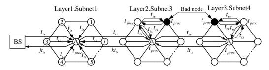
Figure 9. Process of transmission delay with bad node.
