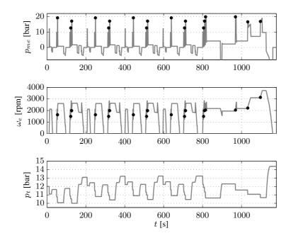
At the end of the drive cycle, the tank pressure is higher by 2.4 bar than at the beginning. Hence, the solution is charge sustaining. The net increase in air-stored  $\Delta M_{a,t}$  amounts to 25 g. The specifications on the pneumatic start mode thus represent a lower boundary on the tank volume because of the high value of  $\tilde{p}_t$ .
