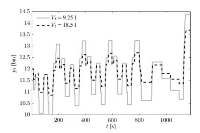
**Figure 9.** Tank pressure trajectories for two different tank volumes.
