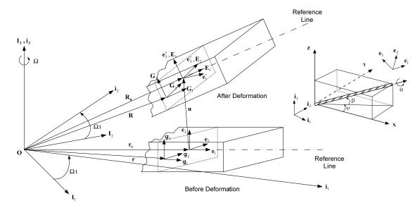
The triad  $\mathbf{e}_1$ ,  $\mathbf{e}_2$  and  $\mathbf{e}_3$  are attached to a reference line along the axis of the deformed blade. The geometrical nonlinearities are described using coordinate transformation matrices with Euler angles, and have the following relationship:
