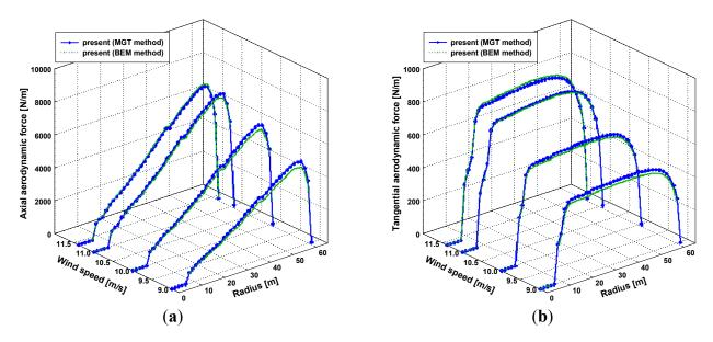
As seen in Figure 9, the close simulation results from both aerodynamic methods were validated in this section. Moreover, fluid-structures analyses were performed to predict the steady-state blade deflections of the NREL 5 MW wind turbine model. A nonlinear beam model, including geometric nonlinearity coupled with the proposed method based on Greenberg's extension of Theodorsen's theory and the BEM method, was employed.
