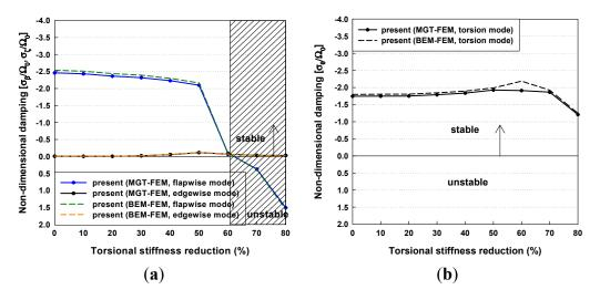
The aeroelastic damping at the cut-out wind speed of 25 m/s is shown in Figure 17, and this had trends similar to the predicted damping at the rated wind speed. The flapwise mode was positively damped above the torsional stiffness reduction of 70%, where the blade is destabilizing. Therefore, it can be concluded that the NREL 5MW wind turbine blade should have at least 40% of the original torsional stiffness applied to prevent dynamic instability under normal operating conditions.
