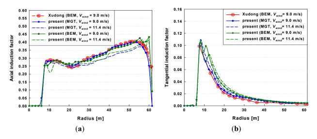
The present results are in relatively good agreement with those presented in the previously published literature [22]. However, small deviations between the present results and the BEM results of [22] were observed at the blade tip because present methods were enhanced with the Prandtl's tip-loss correction, whereas different engineering corrections including tip-loss effect were applied in the previous study [22]. Figure 8 shows the relative velocity and effective angle of attack. The angle of
