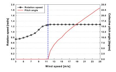
Figure 11. Variations in wind speed versus rotor speed and collective pitch angle.
