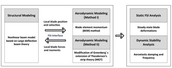
Figure 4. Scheme of fluid-structure interaction analysis for estimating the aeroelastic responses.
