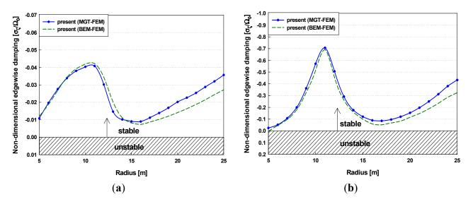
**Figure 13.** Variations in the non-dimensional flapwise damping with wind speed: (**a**) first flapwise mode (1st mode); (**b**) second flapwise mode (3rd mode).
