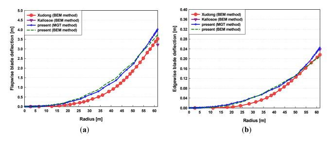
These numerical predictions are highly important for preventing collisions between the rotor blade and tower when MW-sized wind turbines are being developed. Also, the deflections of the blade should be estimated precisely in the design stage because highly deflected blades influence performance, such as the power production.
