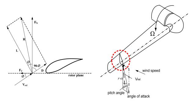
Figure 3. The local normal and tangential loads on a wind turbine blade (BEM method).
