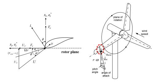
It is assumed that the flow around the pitch regulated wind turbine rotor is incompressible, inviscid, and remains attached to the blade. The pitching moment and aerodynamic forces in normal and tangential directions can be defined as follows:
