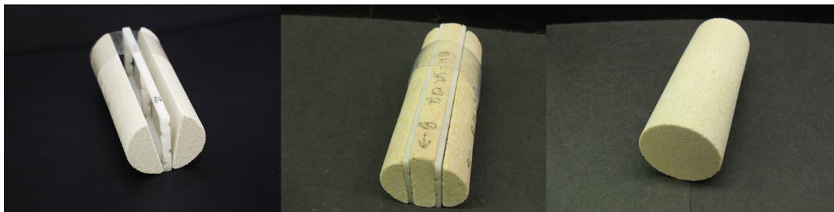
**Figure 4.** Three different core configurations were applied in this study. The fractured design was applied to maximize and provide constant reaction interface while maintaining flow conditions. A double-spacer design was applied to address limitations in diffusion length, while the non-fractured sample was used for more realistic scenarios.
