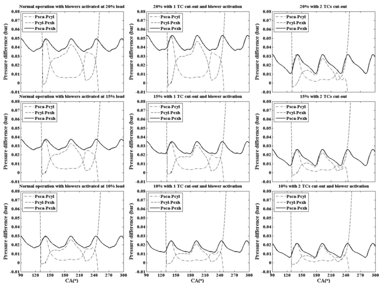
Figure 7. Cylinder pressure difference at different conditions.
