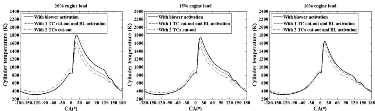
Figure 8. Cylinder temperature at different conditions.
