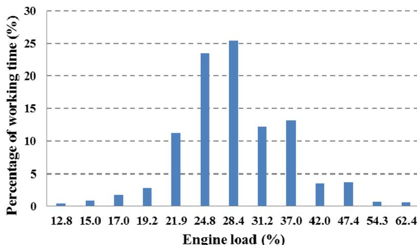
Figure 9. Engine operating profile of panamax vessels in 2012.
