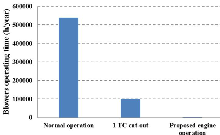
**Figure 11.** Annual blowers operating time (per operating unit); Normal operation: three blowers operate; Operation with 1 TC cut-out: two blowers operate; Proposed engine operation: one blower operates.
