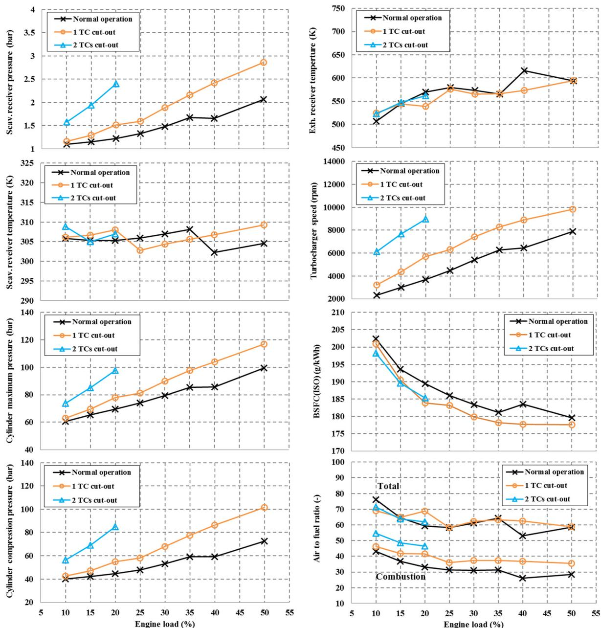
**Figure 6.** Steady state simulation results for normal operation and turbocharger cut-out. (Blowers are activated as follows: below 40% load for normal operation; below 25% load for operation with 1 TC cut-out; at 10% load for operation with 2 TCs cut-out).
