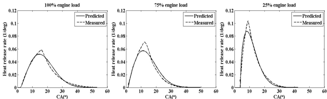
**Figure 2.** Heat release rates at various engine loads.
