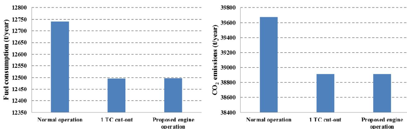
**Figure 10.** Calculated annual fuel consumption (**left**) and CO<sub>2</sub> emissions (**right**).
