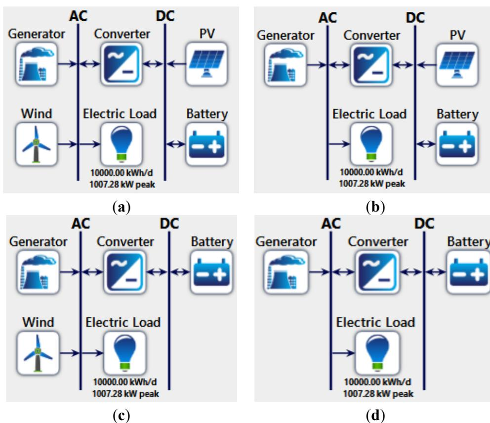
**Figure 7.** (a) Configuration of hybrid PV/wind/diesel/battery system; (b) Configuration of hybrid PV/diesel/battery system; (c) Configuration of hybrid wind/diesel/battery system; (d) Configuration of diesel/battery system.
