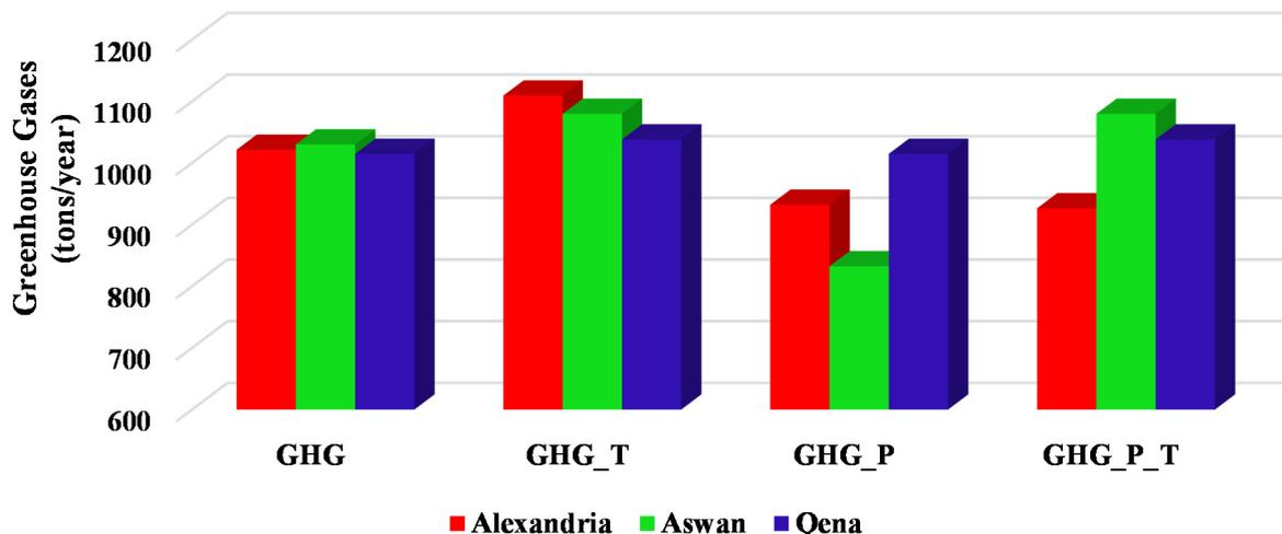
**Figure 12.** The different amounts of GHG emitted from a PV/wind/diesel/battery system in Alexandria, Aswan and Qena.
