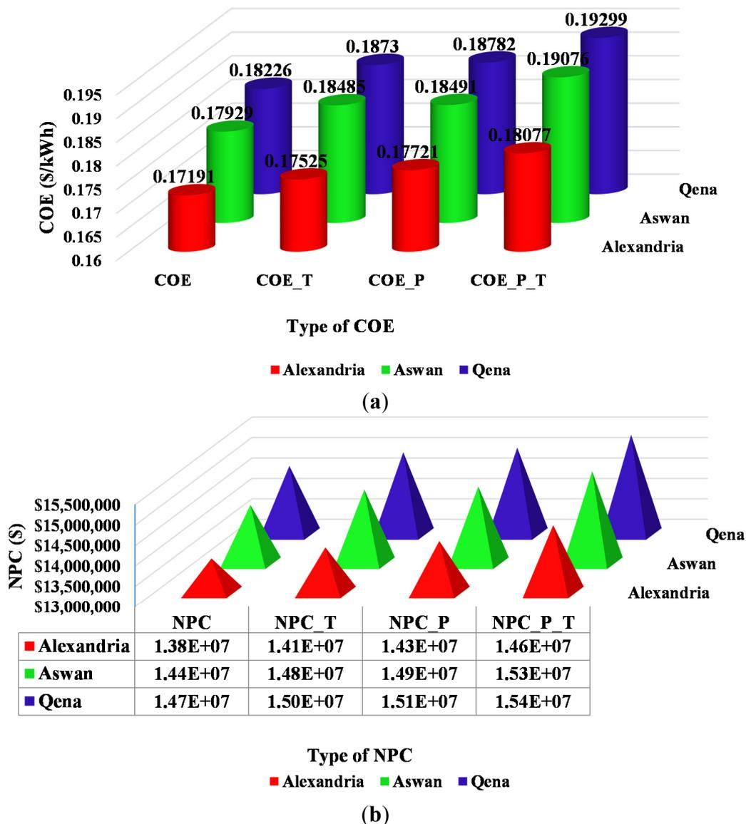
**Figure 8.** (a) The different COE of PV/wind/diesel/battery system in Alexandria, Aswan and Qena; (b) The different NPC of PV/wind/diesel/battery system in Alexandria, Aswan and Qena.
