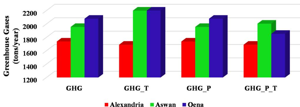
**Figure 14.** The different amounts of GHG emitted from a wind/diesel/battery system in Alexandria, Aswan and Qena.
