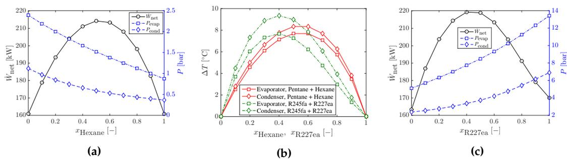
**Figure 2.** Optimal net power-output (maximum  $\dot{W}_{net}$ ) with corresponding operating phase-change pressure, and evaporation and condensation temperature glides at optimal operating conditions. (a) *n*-pentane + *n*-hexane; (b) temperature glides; (c) R-245fa + R-227ea.
