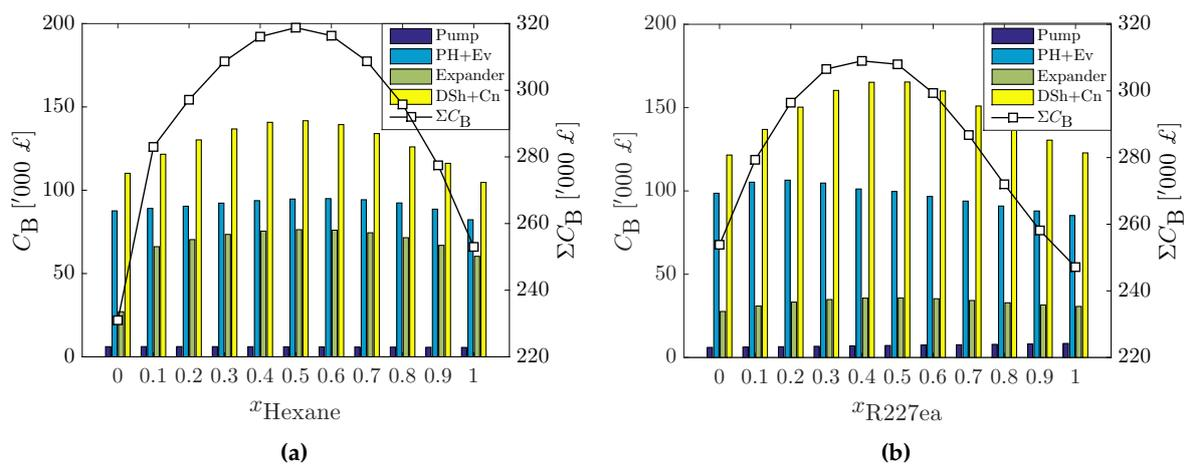
**Figure 7.** Optimal ORC systems' component costs (bars; LHS axes) and total component costs (line; RHS axes). Component-base costs,  $C_B$  are indexed in year 2006, with the following currency conversions: £1  $\equiv$  €1.47, \$1.84. The legend in Figure 7a applies to both figures. (a) *n*-pentane + *n*-hexane; (b) R-245fa + R-227ea.
