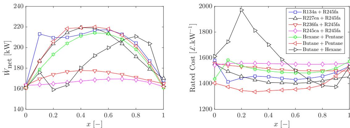
**Figure 8.** Maximum net power output and related rated costs (in pounds per kW) for ORC systems with working fluid mixtures. Cycle heat input is not restricted, *i.e.*,  $\dot{Q}_{in,lim}$  is allowed to attain a maximum possible value; ' $x$ ' represents the mass fraction of the first component fluid in each working-fluid mixture pairing. Component-base costs,  $C_B$ , are indexed in the year 2006, with the following currency conversions: £1  $\equiv$  €1.47, \$1.84.
