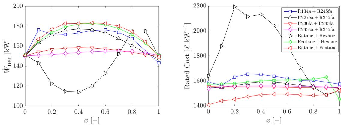
**Figure 9.** Maximum net power output and related rated costs (in pounds per kW) for ORC systems when employing working fluid mixtures. Cycle heat input is restricted to 2.5 MW, *i.e.*,  $Q_{in,lim} = 2.5$  MW; ‘ $x$ ’ represents the mass fraction of the first component fluid in each working-fluid mixture pairing. Component-base costs,  $C_B$ , are indexed in the year 2006, with the following currency conversions:  $\text{£1} \equiv \text{€1.47}$ ,  $\text{\$1.84}$ .
