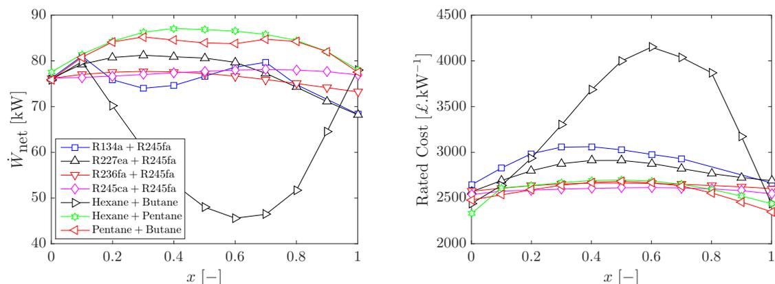
**Figure 10.** Maximum net power output and related rated costs (in pounds per kW) for ORC systems that employ working fluid mixtures. Cycle heat input is restricted to 1.0 MW, *i.e.*,  $Q_{in,lim} = 1.0$  MW; ‘ $x$ ’ represents the mass fraction of the first component fluid in each working-fluid mixture pairing. Component-base costs,  $C_B$ , are indexed in the year 2006, with the following currency conversions:  $\text{£1} \equiv \text{€1.47}$ ,  $\text{\$1.84}$ .
