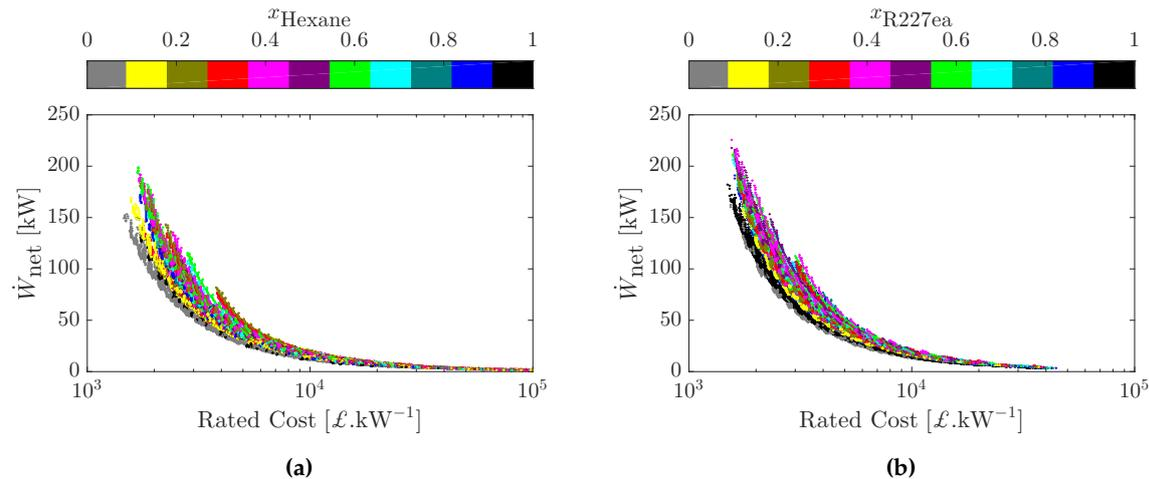
**Figure 11.** The pareto optimal curves for the multi-objective optimization (maximum net power and minimum rated costs in pounds per kW) of ORCs with two sets of working-fluid mixtures. Component-base costs,  $C_B$ , are indexed in the year 2006, with the following currency conversions: £1  $\equiv$  €1.47, \$1.84. (a) *n*-pentane + *n*-hexane; (b) R-245fa + R-227ea.
