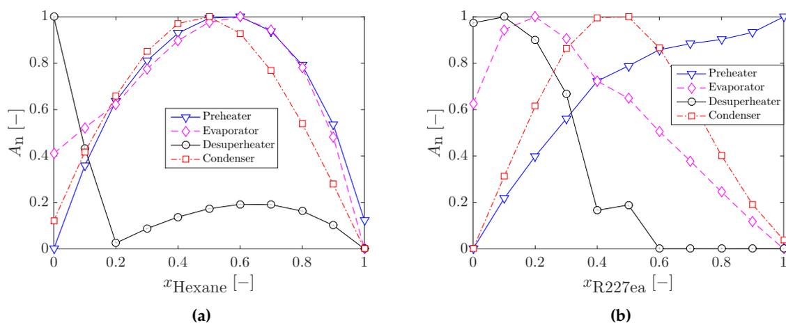
**Figure 6.** Normalized total heat-transfer areas for heat exchangers with the different working-fluid mixtures. Normalization parameters are given in Table 3. (a)  $n$ -pentane +  $n$ -hexane; (b) R-245fa + R-227ea.
