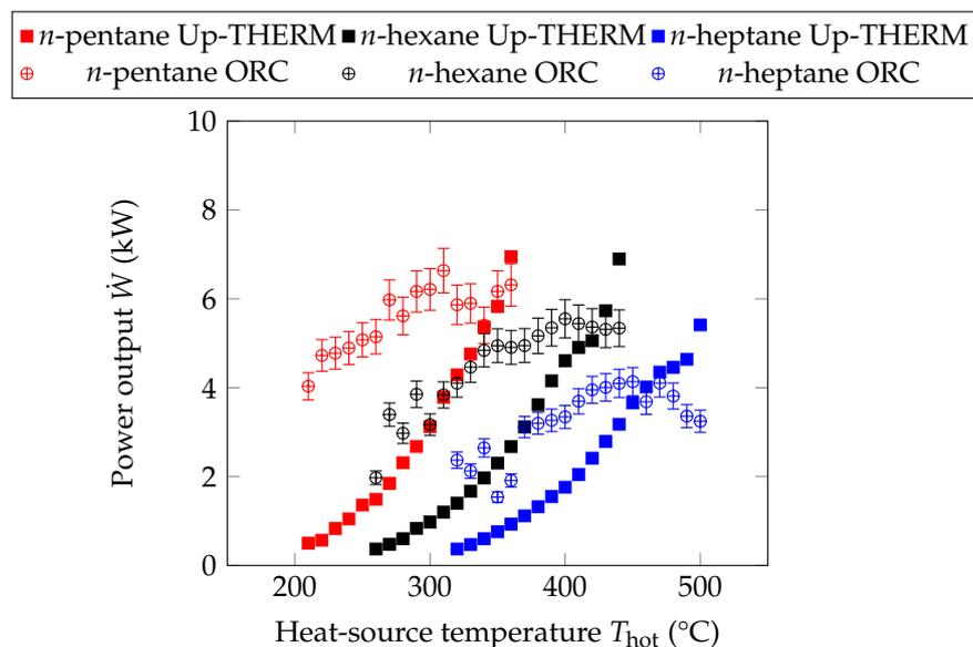
**Figure 5.** Power output from the Up-THERM heat converter and equivalent ORC engines for different working fluids at different heat-source temperatures. For the ORC engines, the circles indicate an expander isentropic efficiency of 0.70 and the error bars isentropic efficiencies of 0.65 and 0.75, respectively.
