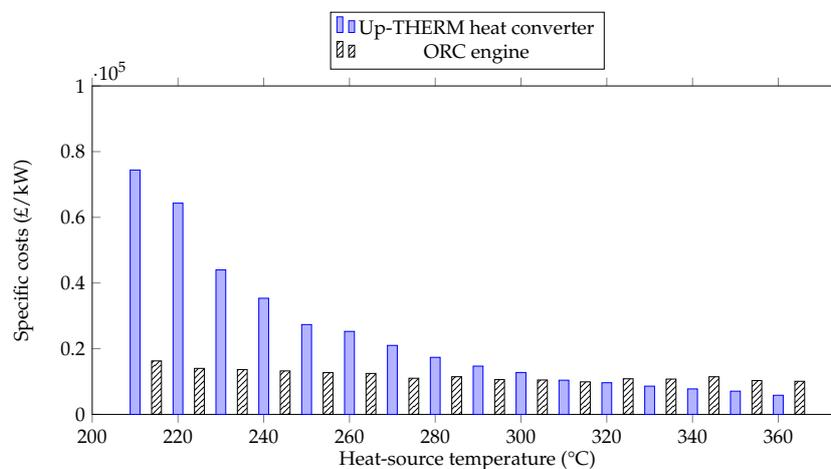
**Figure 12.** Specific costs for the Up-THERM heat converter and equivalent ORC engines for *n*-pentane as the working fluid at different heat-source temperatures.
