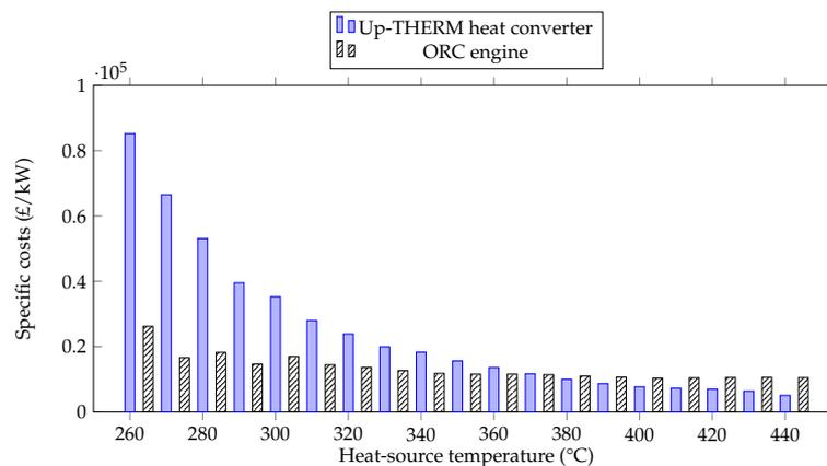
**Figure 13.** Specific costs for the Up-THERM heat converter and equivalent ORC engines for *n*-hexane as the working fluid at different heat-source temperatures.
