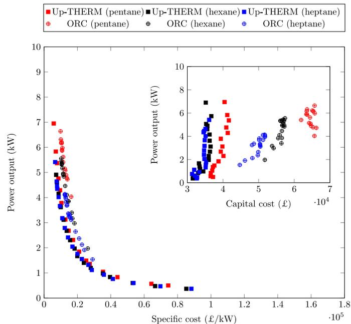
**Figure 16.** Capital cost (inset) and specific cost of the Up-THERM heat converter and ORC engines plotted over the respective power output.
