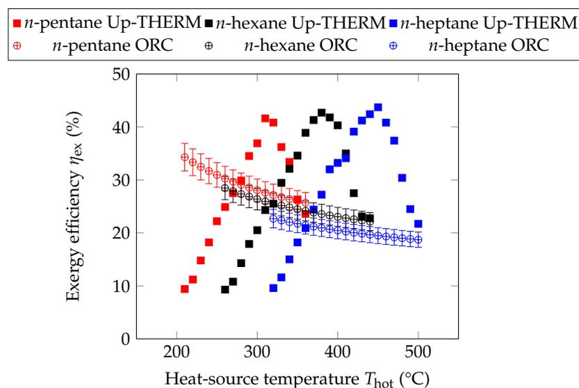
**Figure 6.** Exergy efficiency of the Up-THERM heat converter and equivalent ORC engines for different working fluids at different heat-source temperatures. For the ORC engines, the circles indicate an expander isentropic efficiency of 0.70 and the error bars isentropic efficiencies of 0.65 and 0.75, respectively.
