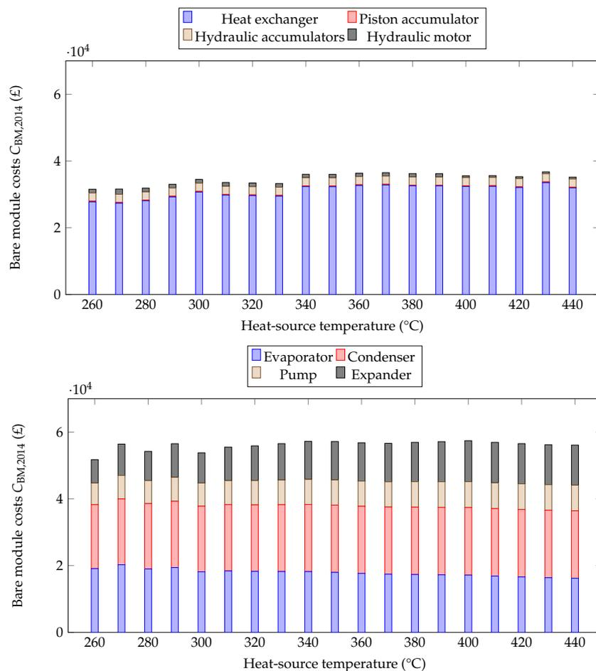
**Figure 9.** Bare module costs for *n*-hexane as the working fluid at different heat-source temperatures: (a) Up-THERM heat converter; and (b) equivalent ORC engines.
