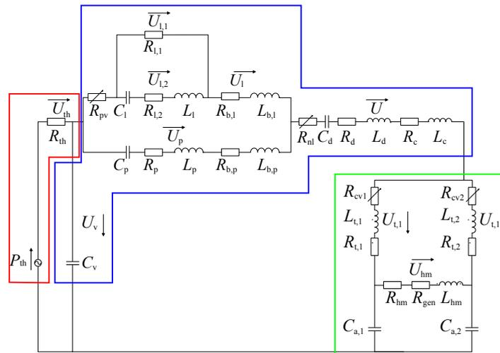
**Figure 3.** Circuit diagram of the Up-THERM engine. The colors represent the same domains (thermal, fluid, and load) of the engine as shown in Figure 1.
