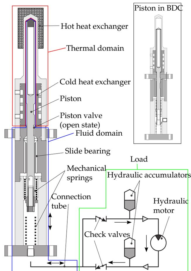
**Figure 1.** Schematic of the Up-THERM heat engine with hot heat-exchanger (HHX) and cold heat-exchanger (CHX), piston, piston valve, mechanical spring and hydraulic motor with piston at top dead centre (TDC) and bottom dead centre (BDC, inset).
