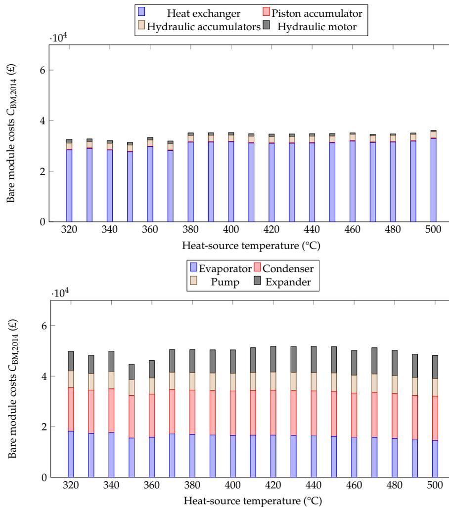
**Figure 10.** Bare module costs for *n*-heptane as the working fluid at different heat-source temperatures: (a) Up-THERM heat converter; and (b) equivalent ORC engines.
