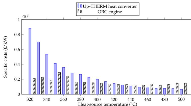
**Figure 14.** Specific costs for the Up-THERM heat converter and equivalent ORC engines for *n*-heptane as working fluid at different heat-source temperatures.
