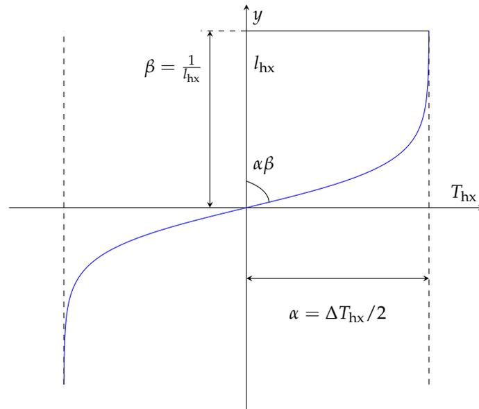
**Figure 2.** Non-linear temperature profile along the inner surfaces of the heat-exchanger walls, showing a temperature saturation at long lengths from the origin (equilibrium position mid-way between the hot and cold heat exchangers).
