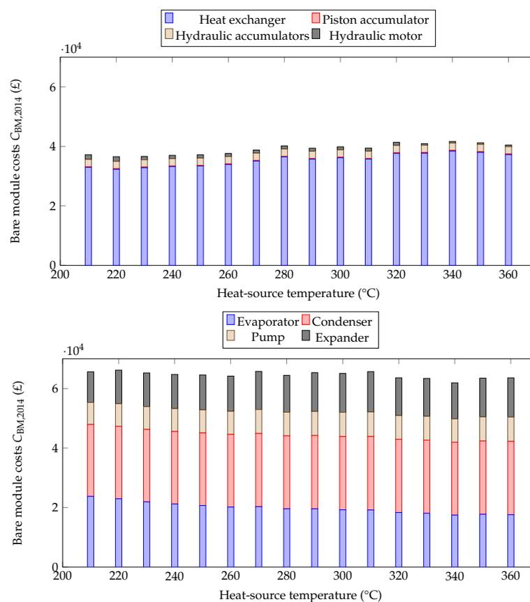
**Figure 8.** Bare module costs for  $n$ -pentane as the working fluid at different heat-source temperatures: (a) Up-THERM heat converter; and (b) equivalent ORC engines.
