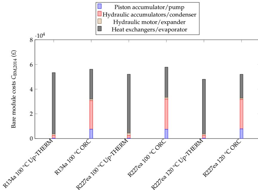
**Figure 11.** Bare module costs for the Up-THERM heat converter and equivalent ORC engines for the refrigerants R134a and R227ea as working fluids at different heat-source temperatures.
