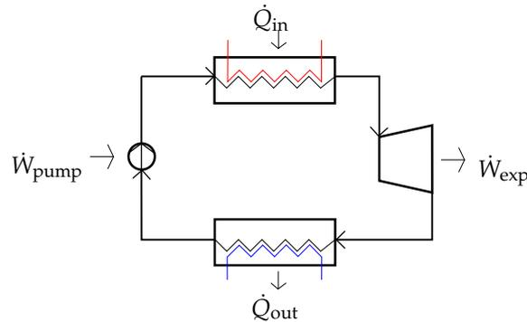
Figure 4. Schematic of the sub-critical organic Rankine cycle (ORC) engine.
