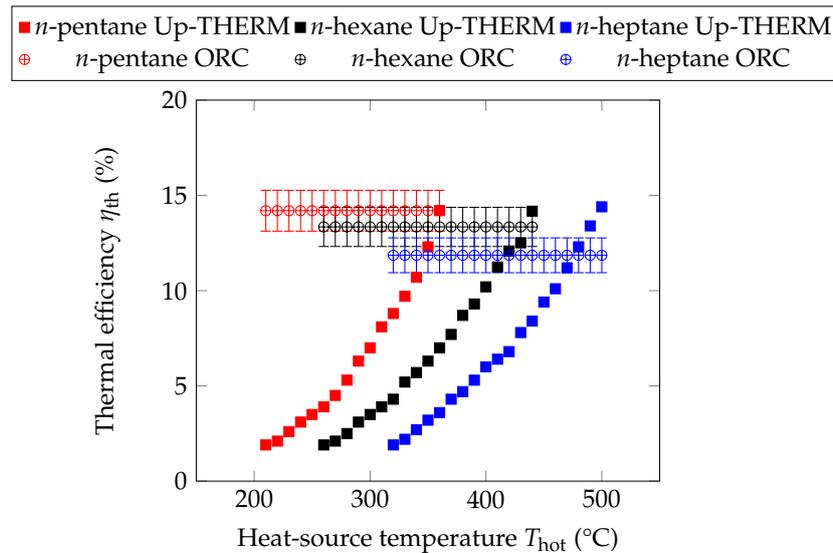
**Figure 7.** Thermal efficiency of the Up-THERM heat converter and equivalent ORC engines for different working fluids at different heat-source temperatures. For the ORC engines, the circles indicate an expander isentropic efficiency of 0.70 and the error bars isentropic efficiencies of 0.65 and 0.75, respectively.
