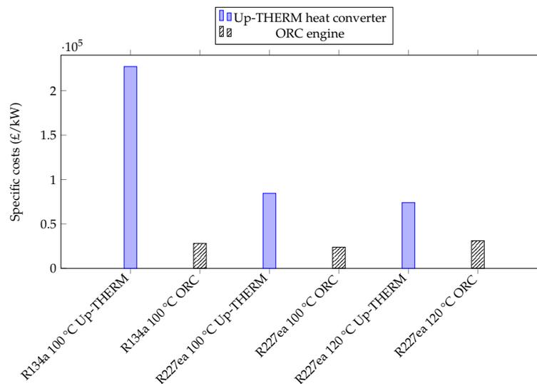
**Figure 15.** Specific costs for the Up-THERM heat converter and equivalent ORC engines for R134a and R227ea as working fluids at different heat-source temperatures.
