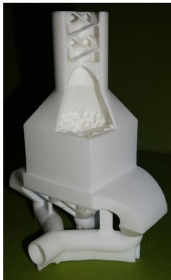
**Figure 6.** Alumina static mixer additively manufactured by lithography-based ceramic manufacturing (LCM) at Fraunhofer IKTS.
