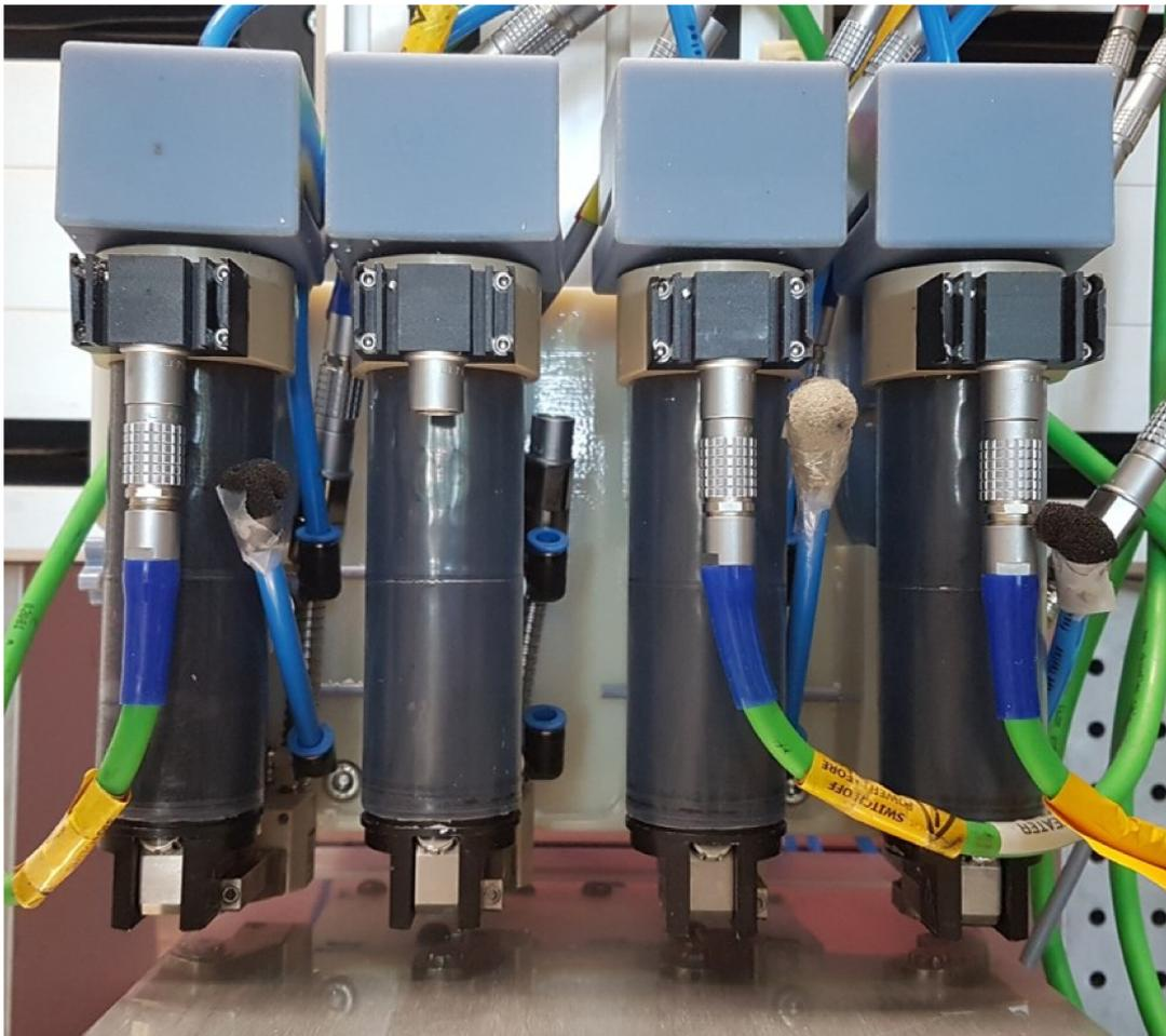
**Figure 8.** Thermoplastic 3D printing (T3DP) device with four different micro dispensing units.
