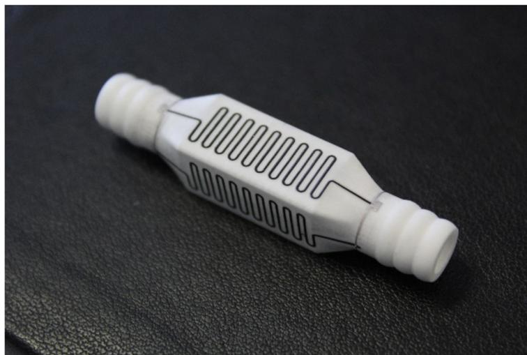
**Figure 7.** Post-functionalized additively manufactured alumina component (Fraunhofer IKTS).
