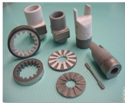
**Figure 1.** Metal–ceramic composites manufactured by two-component ceramic injection molding (2C-CIM) (manufactured by group “Shaping” at FhG-IKTS).
