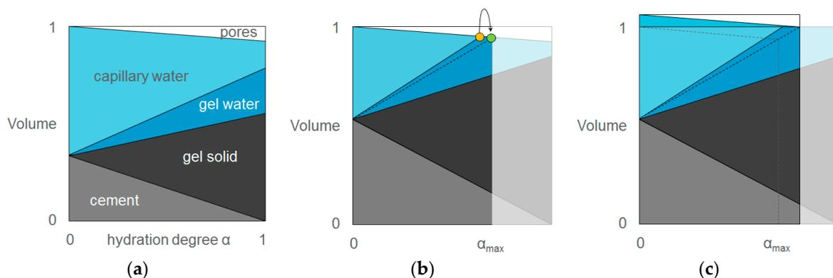
**Figure 3.** Principle of autogenous shrinkage in a system with a high water-to-cement ratio (a), and a low water-to-cement ratio without (b) and with internal curing (c).
