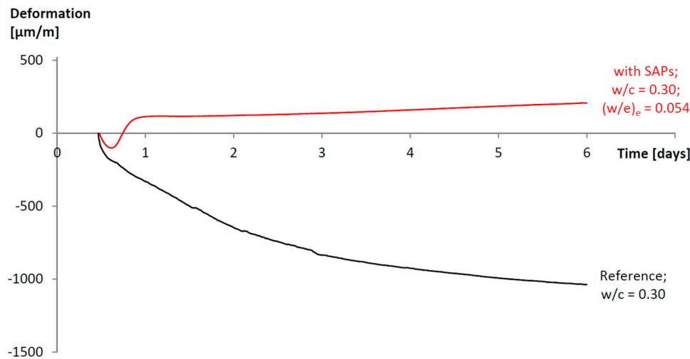
**Figure 4.** Mitigation of the autogenous shrinkage in a cementitious system with a water-to-cement ratio of 0.30 by means of superabsorbent polymer inclusion. Adapted from [17,78], with permission from © 2015 Elsevier.
