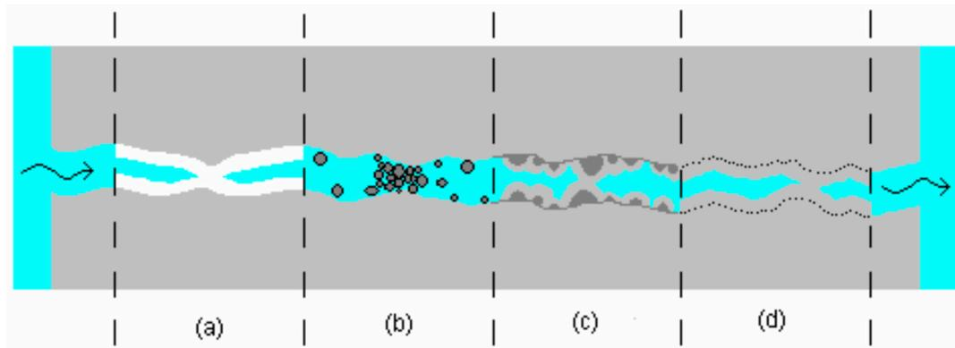
**Figure 7.** Different mechanisms of autogenous healing: (a) the deposition of  $\text{CaCO}_3$  or  $\text{Ca}(\text{OH})_2$  crystals; (b) filling of the crack by pollutants in the water and loose concrete particles from spalling; (c) formation of new silicates by hydration of unreacted cement particles near the edge of the fracture and (d) expansive reaction of the hydrated cementitious matrix [163].
