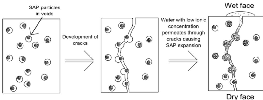
**Figure 5.** Schematic display of self-sealing of cracks in concrete by using SAPs. Adapted from [146], with permission from © 2010 Taylor & Francis.
