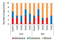
Figure S1. Fracture modes obtained from the push-out bond testing.
