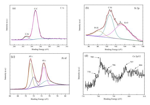
Figure 9. XPS spectra of the Pt<sub>3</sub>Co–SiC nanowires: (a) C 1s; (b) Si 2p; (c) Pt 4f; (d) Co 2p3/2.
