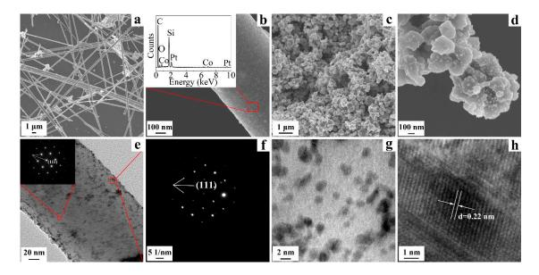
**Figure 3.** SEM images of Pt<sub>3</sub>Co-SiC nanowires (**a**,**b**); Pt<sub>3</sub>Co-SiC powders (**c**,**d**); TEM images of Pt<sub>3</sub>Co-SiC nanowires (**e**,**f**); Pt<sub>3</sub>Co-SiC powders (**g**,**h**).
