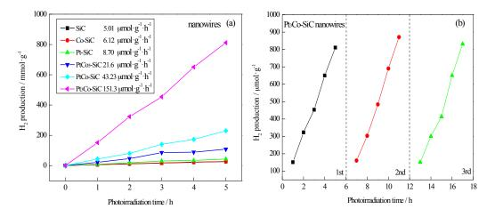
**Figure 5.** (a) Photocatalytic hydrogen evolution performance over: Pt<sub>3</sub>Co-SiC, PtCo-SiC, PtCo<sub>3</sub>-SiC, Pt-SiC, Co-SiC, SiC; (b) cyclic experiments of Pt<sub>3</sub>Co-SiC nanowire over water splitting.
