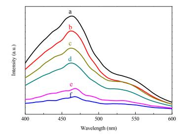
Figure 7. PL spectra of SiC (a); Co-SiC (b); Pt-SiC (c); PtCo<sub>3</sub>-SiC (d); PtCo-SiC (e); Pt<sub>3</sub>Co-SiC (f).
