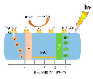
Figure 10. Schematic diagram of photocatalytic mechanism for H<sub>2</sub> production over Pt<sub>3</sub>Co-SiC.
