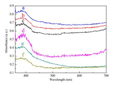
Figure 6. UV-Vis diffusion reflectance spectra of Pt<sub>3</sub>Co-SiC (a); PtCo-SiC (b); PtCo<sub>3</sub>-SiC (c); Pt-SiC (d); Co-SiC (e); SiC (f).
