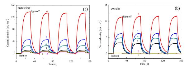
**Figure 4.** Current density of the different SiC nanowires photoelectrode: Pt<sub>3</sub>Co-SiC (6), PtCo-SiC (5), PtCo<sub>3</sub>-SiC (4), Pt-SiC (3), Co-SiC (2), SiC (1) at open circuit voltage in the dark and simulated solar light (a); different SiC powders photoelectrode: Pt<sub>3</sub>Co-SiC (6), PtCo-SiC (5), PtCo<sub>3</sub>-SiC (4), Pt-SiC (3), Co-SiC (2), SiC (1) at open circuit voltage in the dark and simulated solar light (b).
