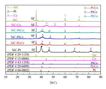
**Figure 2.** XRD and corresponding PDF standard patterns of the pure SiC powders, and SiC powders loaded with Pt-Co alloy.
