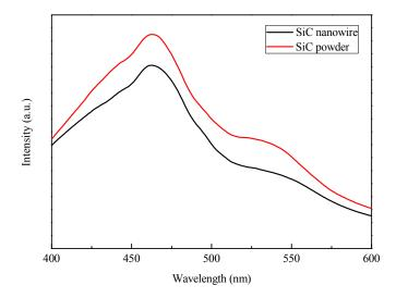
Figure 8. PL spectra of SiC powder and SiC nanowire.
