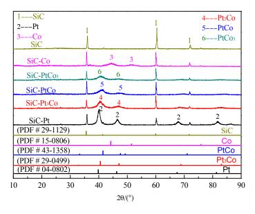
**Figure 1.** X-ray diffraction (XRD) and corresponding PDF standard patterns of the pure SiC nanowires, and SiC nanowires loaded with Pt-Co alloy.
