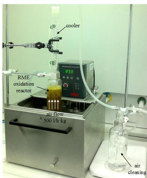
**Figure 1.** Laboratory setup for bio-agent production: reactor for oxidation of rapeseed oil esters.
