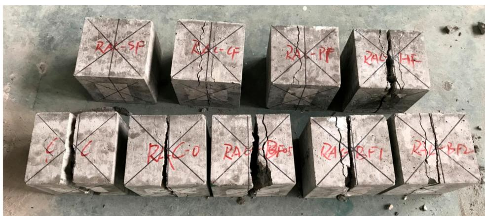
**Figure 8.** Failure modes of splitting tensile specimens.
