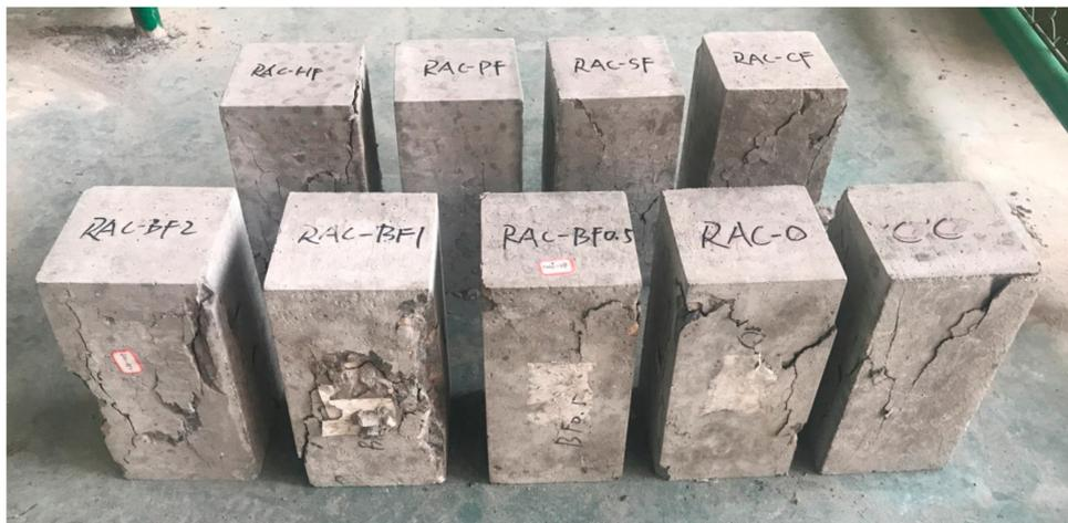
**Figure 6.** Failure modes of axial compressive specimens.
