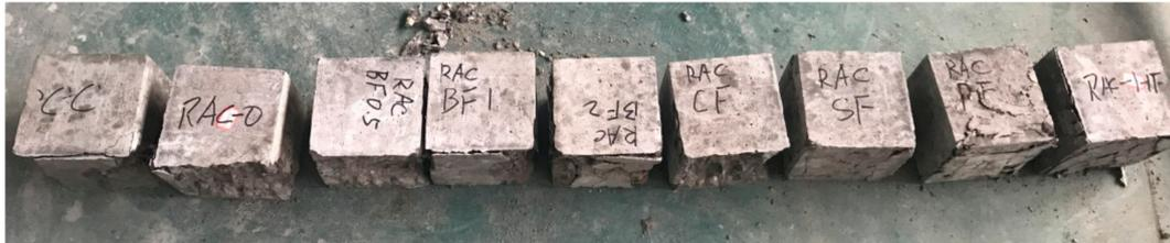
**Figure 5.** Failure modes of cube compressive specimens.
