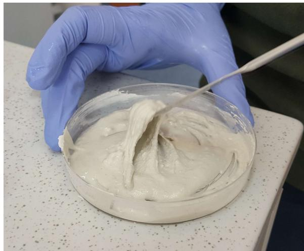
**Figure 3.** Chewing gum-like consistency of P50 samples after mixing of bioceramic and polymeric components.
