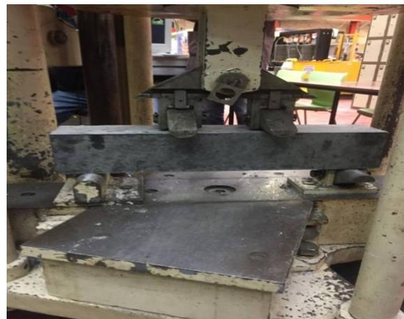
Figure 10. 4-point bending test.
