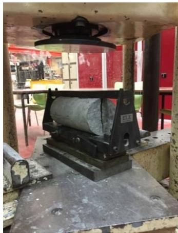
Figure 9. Splitting tensile test.
