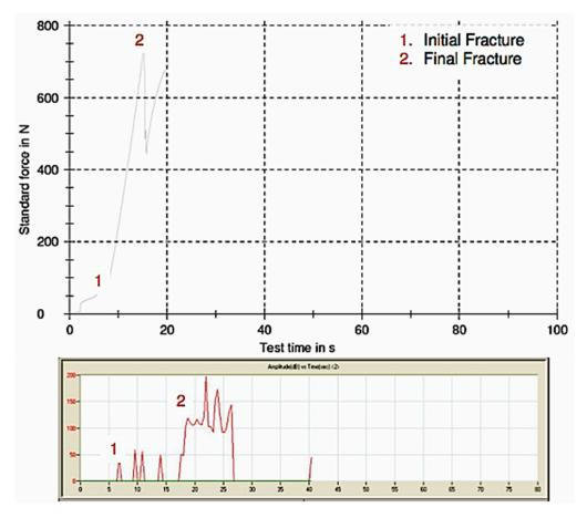
**Figure 2.** Graphs of the load-time relationship and amplitude-time relationship produced by the Zwick and AE sensor respectively.
