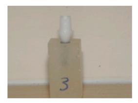
Figure 1. Implant-abutment assembly mounted on acrylic blocks.
