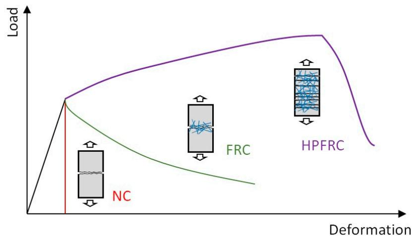
**Figure 1.** Tensile stress deformation behavior of normal concrete (NC), fiber-reinforced concrete (FRC), and high-performance fiber-reinforced concrete (HPFRC) [11–13].
