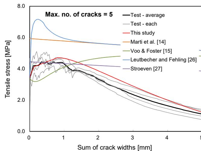
**Figure 11.** Comparison with FRC tension models.
