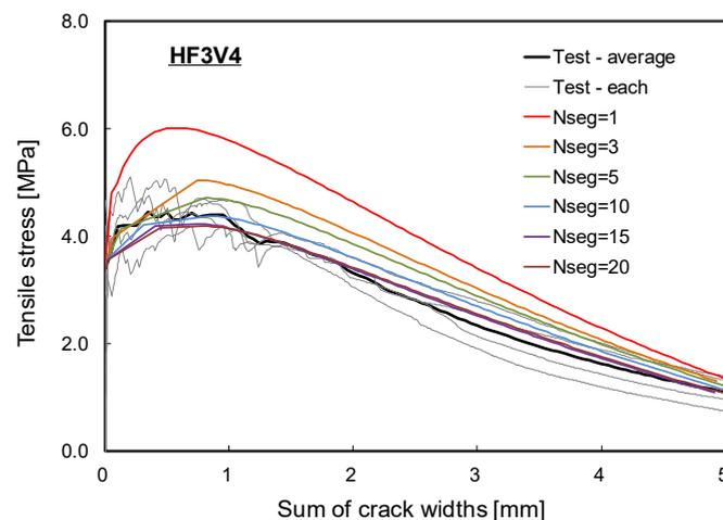
Figure 10. Comparison of the prediction and the test results for the tensile behavior.
