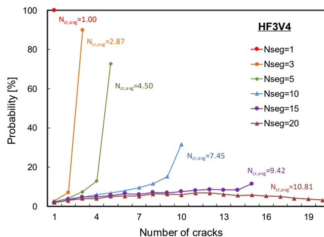
Figure 9. Probabilistic distribution on the predicted number of cracks.
