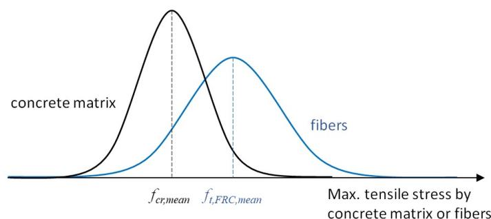
Figure 7. Normal distribution of the tensile stress due to steel fibers.
