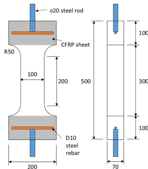
Figure 8. Details of the specimens tested by Lee et al. [20].
