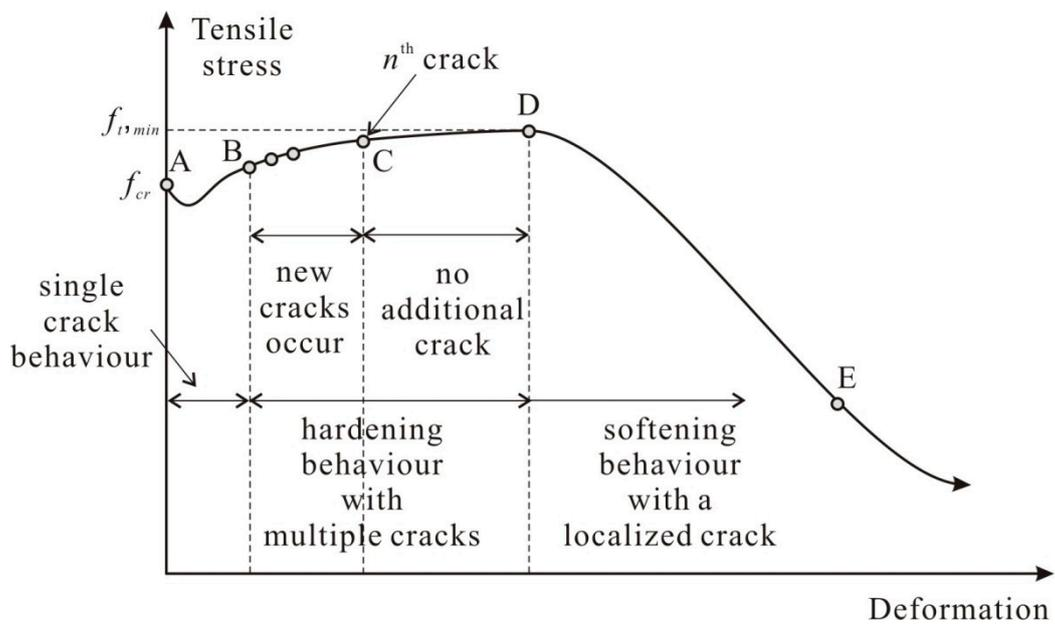
**Figure 3.** Tensile stress-deformation response in HPFRC.
