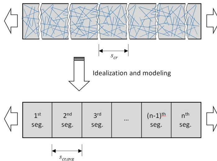
Figure 6. Analytical model with segments for an HPFRC member subjected to uniaxial tension.
