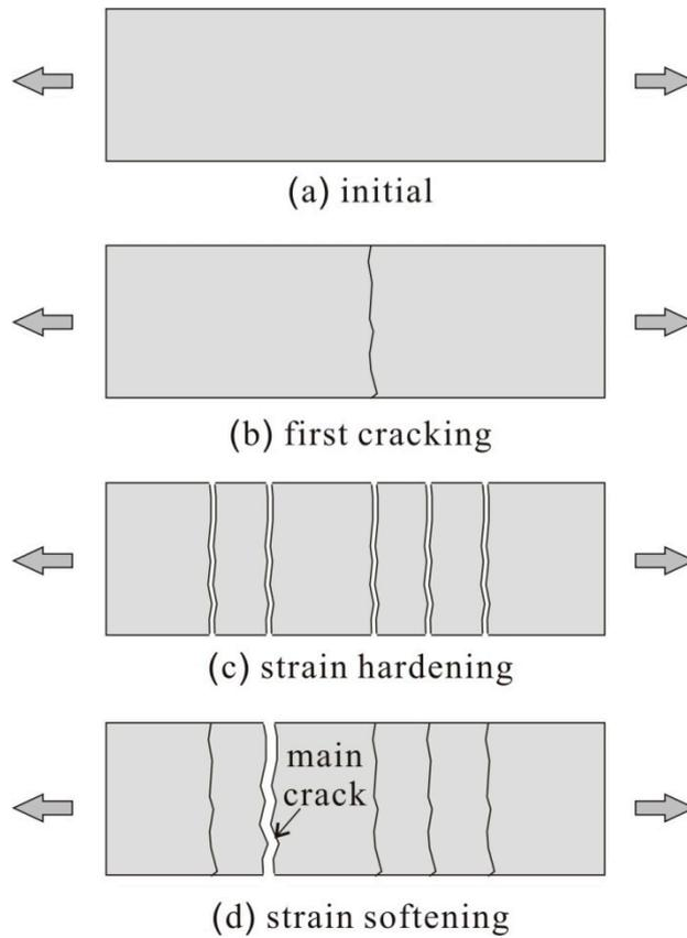
**Figure 2.** Cracking pattern of HPFRC subjected to tension. (a) initial; (b) first cracking; (c) strain hardening; (d) strain softening.
