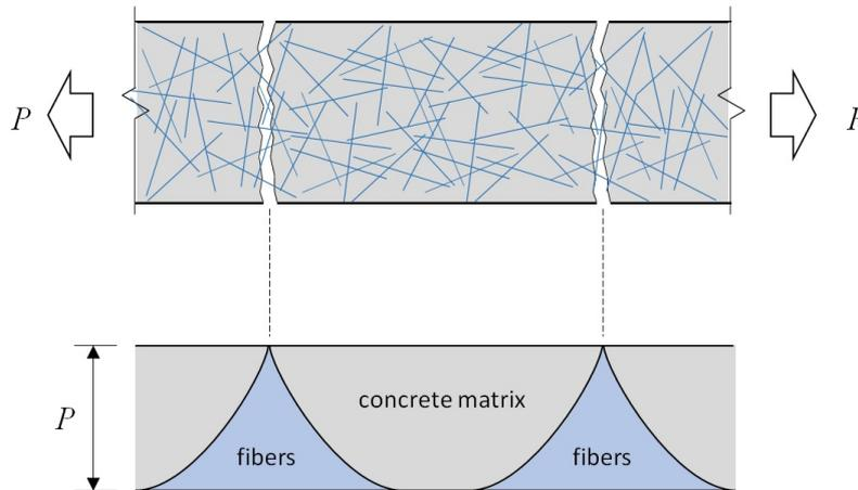
Figure 5. Concrete matrix and steel fiber tensile stress distributions between cracks.
