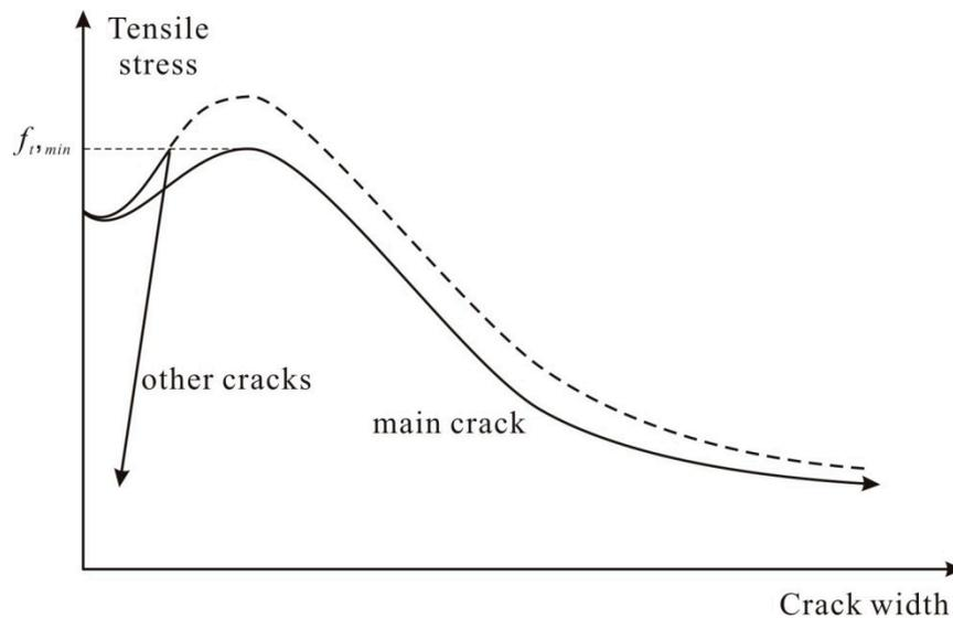
Figure 4. Tensile stress-crack width opening response at the main crack and the others.
