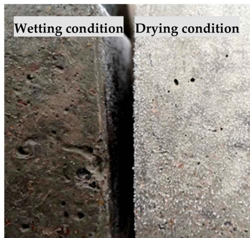
**Figure 4.** Comparison of salt crystal distribution on concrete surface between wetting and drying conditions.
