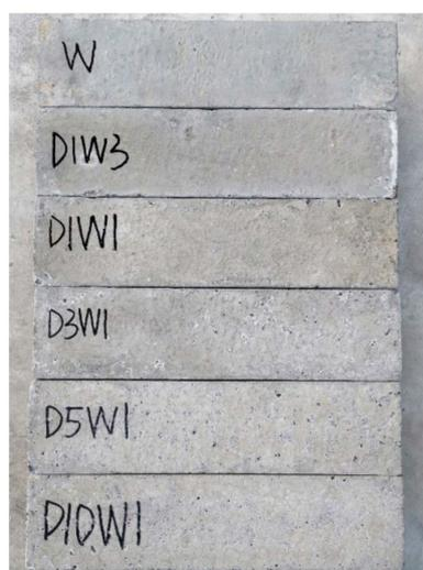
**Figure 3.** Visual inspection of concrete exposed to sulfate solution under drying–wetting cycles.
