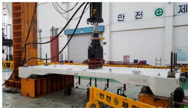
**Figure 9.** Fatigue testing of SC120f-PSC-JF specimen.
