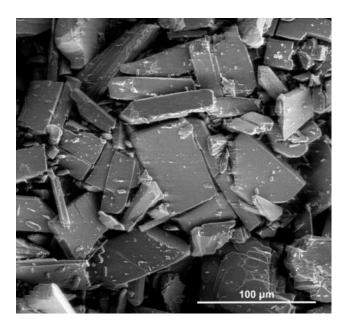
$\textbf{Figure S7.} \ SEM \ image \ of \ commercial \ NH_4VO_3 \ used \ in \ a \ hydrothermal \ synthesis.$
