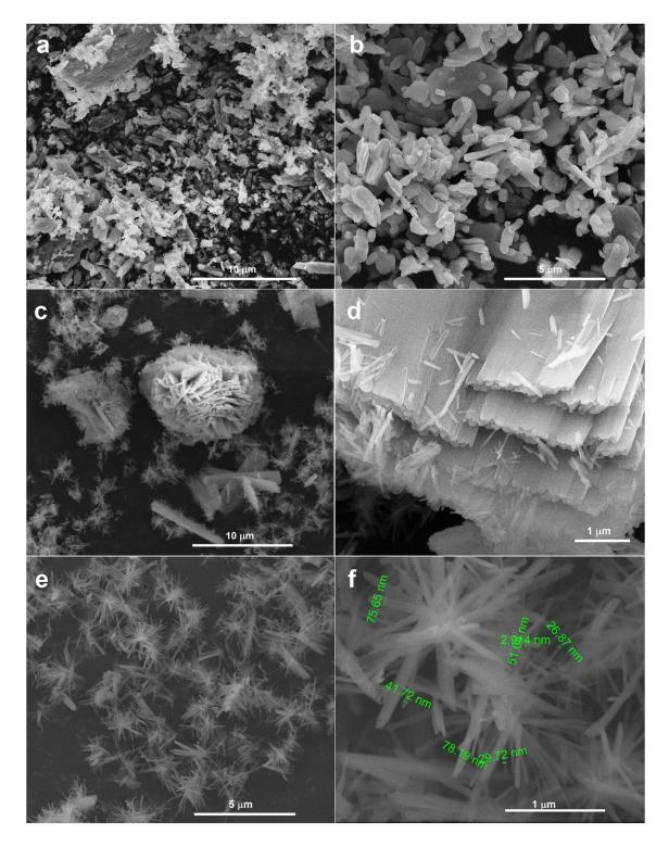
**Figure S3.** SEM images presenting the structure of  $V_2O_5$  used as a precursor (a,b) and intermediates formed in the reaction of  $V_2O_5$  with ammonium formate in formamide (c,d), leading to flower-like nanostructural crystals of NH<sub>4</sub>VO<sub>3</sub> (e,f).
