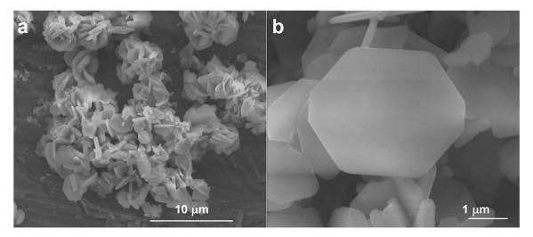
**Figure S6.** SEM images presenting structures of NH<sub>4</sub>VO<sub>3</sub> obtained in the reaction of  $V_2O_5$  and ammonium formate carried out in the 1:1 (v/v) mixture of water and formamide.
