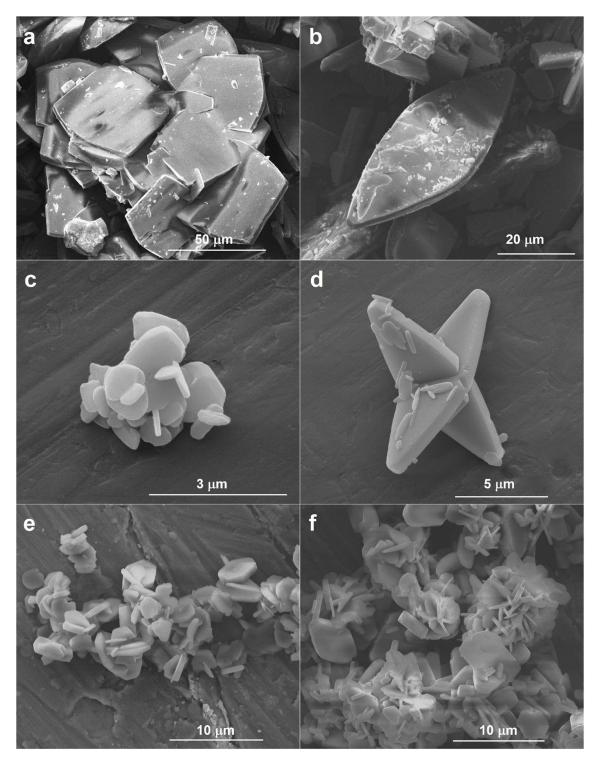
**Figure S4.** SEM images presenting structures of NH<sub>4</sub>VO<sub>3</sub> obtained from  $V_2O_5$  in water using ammonium formate (**a**,**b**), ammonium acetate (**c**,**d**), and equimolar mixture of ammonium formate and ammonium acetate (**e**,**f**).
