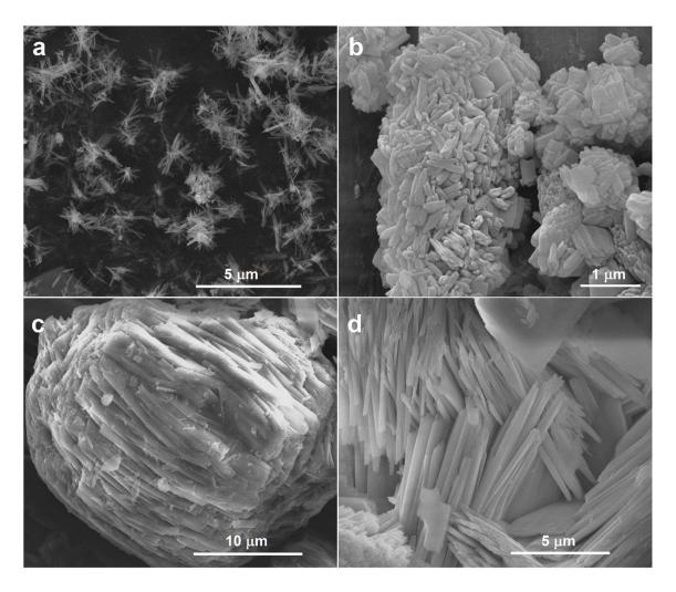
**Figure S5.** SEM images presenting structures of NH<sub>4</sub>VO<sub>3</sub> obtained from  $V_2O_5$  in formamide using ammonium formate (a), ammonium acetate (b), and equimolar mixture of ammonium formate and ammonium acetate (c,d).
