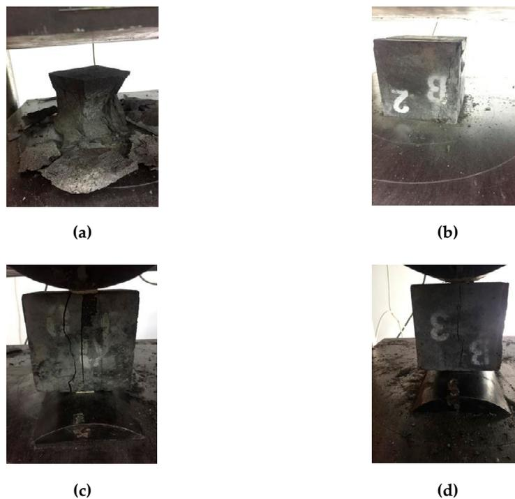
**Figure 8.** Influence of steel fiber on the mechanical properties of RPC: (a) compressive damage without steel fiber; (b) compressive damage with steel fiber; (c) split tensile failure without steel fiber; (d) split tensile failure with steel fiber.
