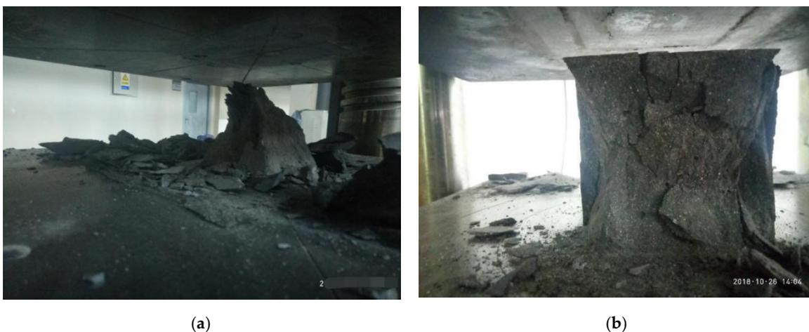
Figure 3. Compression failure morphology: (a) reactive powder concrete (RPC), (b) carbon-fiber RPC.
