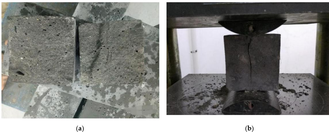
**Figure 6.** Splitting tensile failure morphology: (a) RPC, (b) carbon-fiber RPC.
