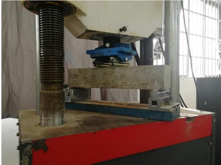
Figure 4. Flexural test.
