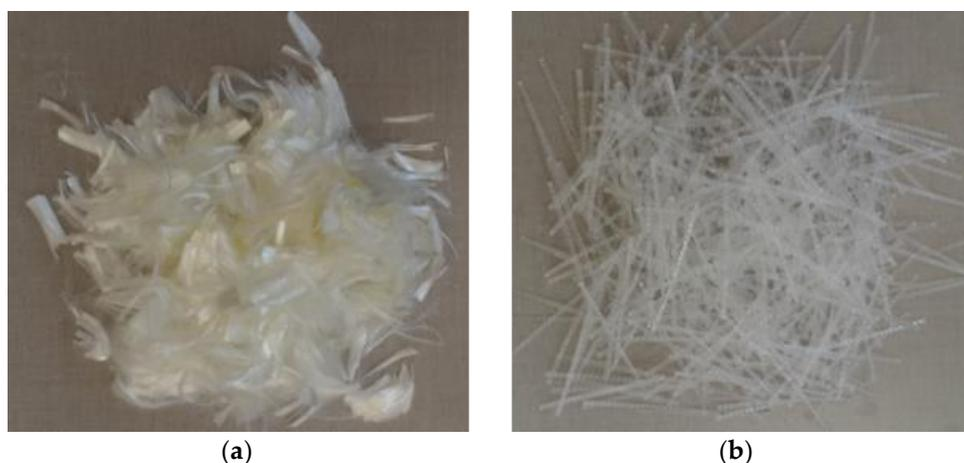
**Figure 1.** Appearance of fibers: (a) Polyvinyl alcohol fibers (PVAf); (b) Polypropylene plastic steel fibers (PPSF).
