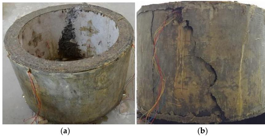
**Figure 9.** Failure characteristic of D-0 model specimen (reference concrete): (a) failure characteristic of inside surface (b) failure characteristic of outside surface.
