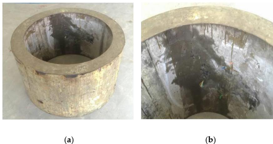
**Figure 10.** Failure characteristic of D-1 model specimen (HFRC): (a) an intact whole, (b) micro-cracks.
