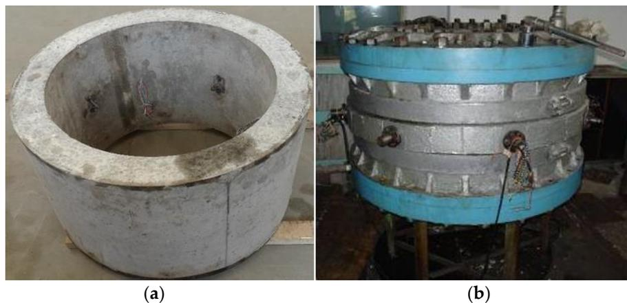
Figure 5. Analog simulation model test: (a) Model specimen; (b) High-pressure loading device.
