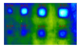
Figure 15. Delaminations (B-D1 to B-D8) on thermal image at 11:30 on day 1.
