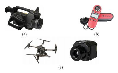
Figure 9. Equipment used in the experiment: (a) H-IRC; (b) Kestrel 3000; (c) UAV-IRC.
