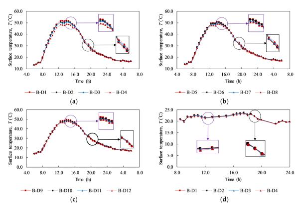
**Figure 12.** Surface temperature above delaminations: (**a**) at 2 cm depth on day 1; (**b**) at 3 cm depth on day 1; (**c**) at 4 cm depth on day 1; (**d**) at 2 cm depth on day 2.
