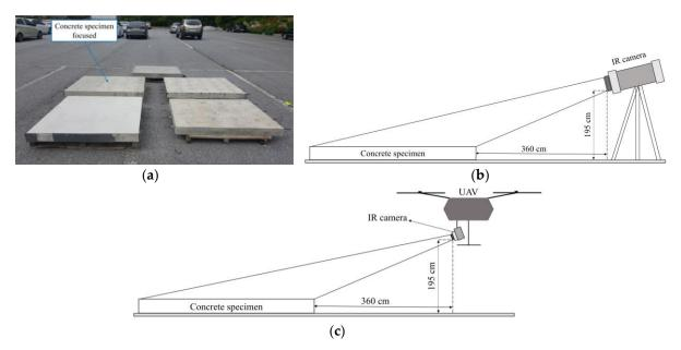
Figure 8. Arrangement of the experiment: (a) location of specimen; (b) with H-IRC; (c) with UAV-IRC.
