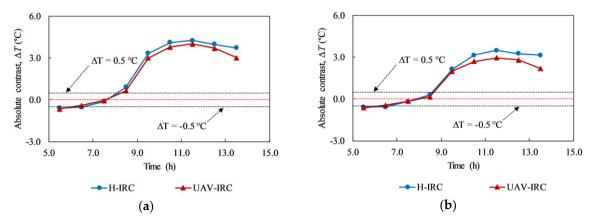
**Figure 22.** Comparison between the absolute contrast captured by H-IRC and UAV-IRC on a sunny day (day 5): (a) delamination B-D2; (b) delamination B-D5.
