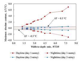
**Figure 17.** Maximum absolute contrast of delaminations during daytime and nighttime on both days 1 and 2.
