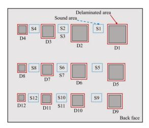
Figure 13. Selection of delaminated and sound areas on the structure surface.
