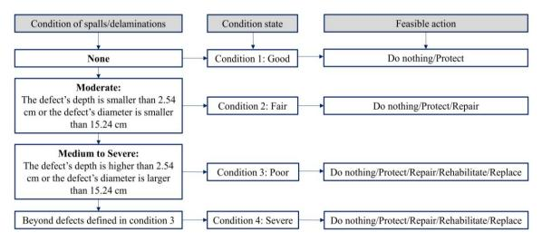
**Figure 2.** Classification of concrete bridge deck conditions required by American Association of State Highway and Transportation Officials (AASHTO) 2015.
