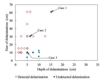
Figure 3. Detected and undetected delaminations summarized from the literature.
