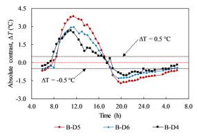
Figure 16. Absolute contrasts of delaminations with different WTDRs on day 1.
