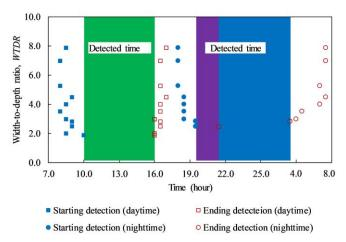
Figure 19. Feasible time on a sunny day to detect delamination in concrete bridge deck.
