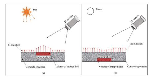
Figure 4. Fundamentals of defect detection using passive IRT: (a) during daytime; (b) during nighttime.
