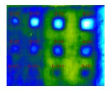
Figure 20. Thermal image of specimen surface using UAV-IRC at 11:30.
