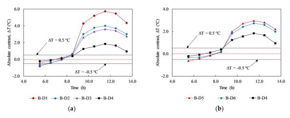
**Figure 21.** Absolute contrast of delaminations with different WTDRs on day 5 from UAV-IRC: (a) at same depth of 2 cm; (b) at different depths of 2 and 3 cm.
