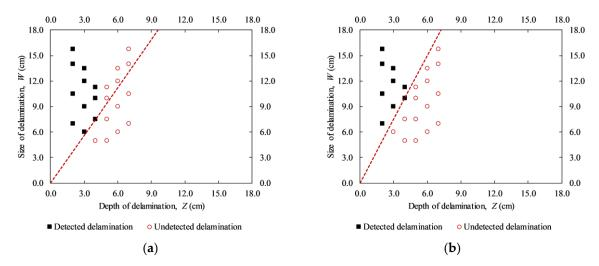
**Figure 18.** Detected and undetected delaminations on the sunny day (day 1 and day 3): (a) daytime; (b) nighttime.
