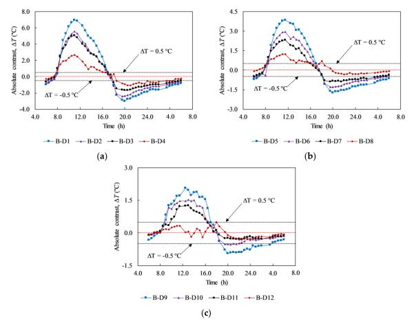
**Figure 14.** Absolute contrast of delaminations with different depths and sizes on day 1: (a) at the depth of 2 cm; (b) at the depth of 3 cm; (c) at the depth of 4 cm.
