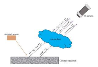
Figure 5. Radiation received by an infrared (IR) camera.
