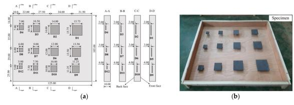
**Figure 6.** Concrete specimen with embedded imitating delaminations: (a) arrangement of delaminations; (b) formwork to cast the concrete specimen.
