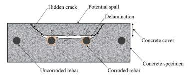
Figure 1. Locations of delaminations in concrete structure.
