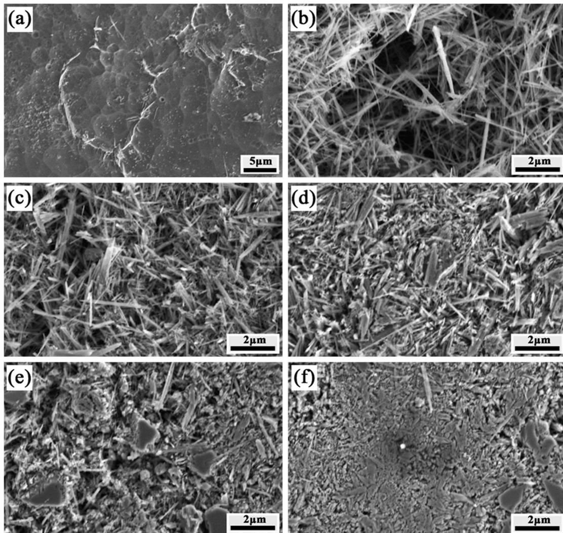
**Figure 3.** Micrographs of layers 1-6 of temperature gradient field sintering. (a) layer 1, (b) layer 2, (c) layer 3, (d) layer 4, (e) layer 5 and (f) layer 6.
