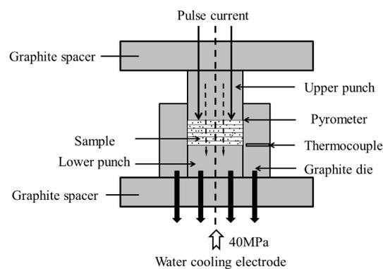
**Figure 2.** Schematic diagram of temperature gradient field (TGF) sintering by spark plasma sintering (SPS).
