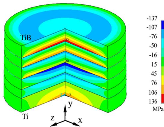
Figure 4. 3-D Geometrical model and residual stress distribution of the Ti-TiB-TiB<sub>2</sub> FGM.
