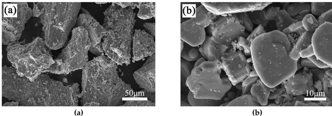
Figure 1. SEM micrographs of original powder particles of Ti (a) and TiB<sub>2</sub> (b).
