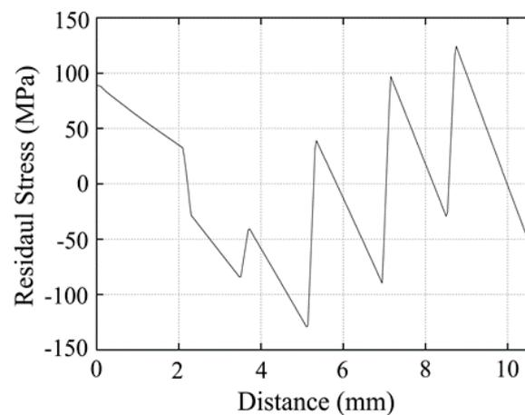
Figure 5. Calculated axial stress in the direction of the radial centre of the FGM sintered by TGF.
