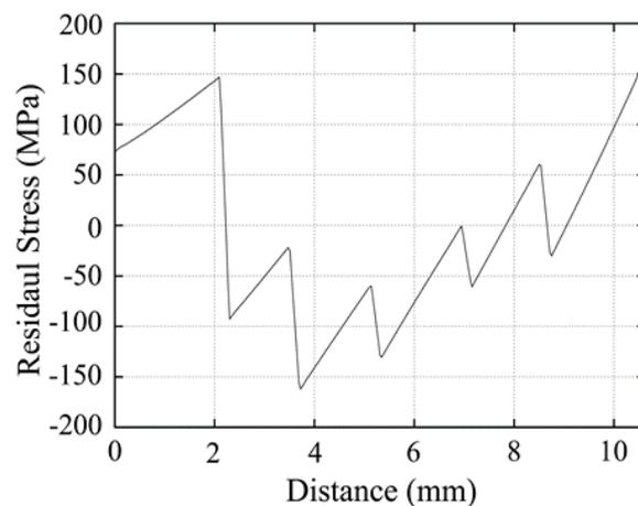
Figure 6. Calculated axial stress in the direction of the radial centre of the FGM uniformly sintered at 1100 °C.
