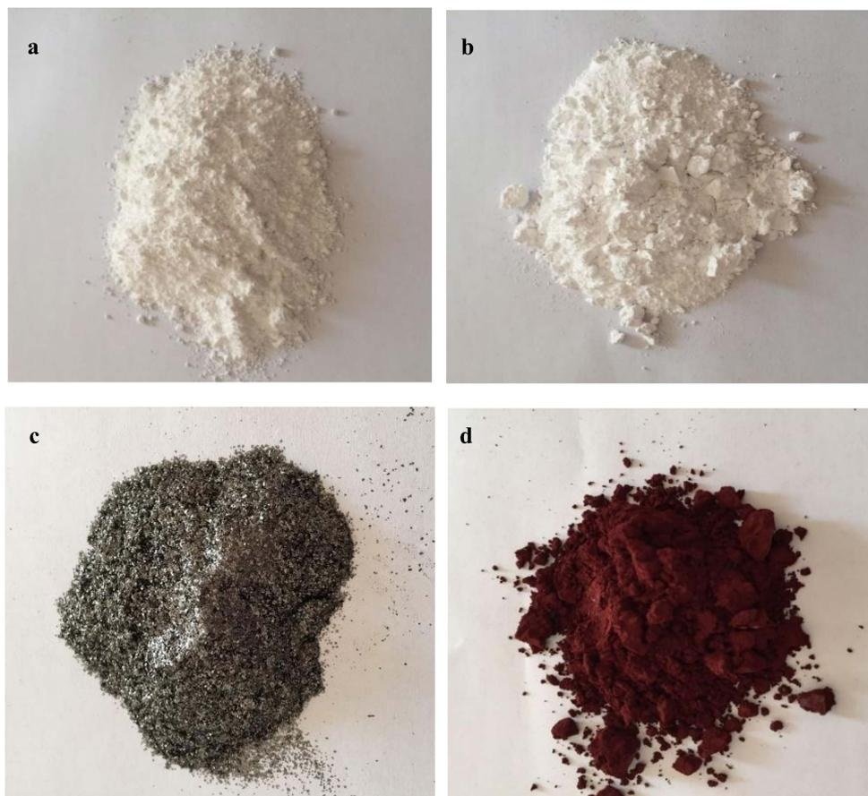
**Figure 1.** Four fire retardants. (a) Aluminum hydroxide; (b) magnesium hydroxide; (c) expanded graphite; (d) encapsulated red phosphorous.
