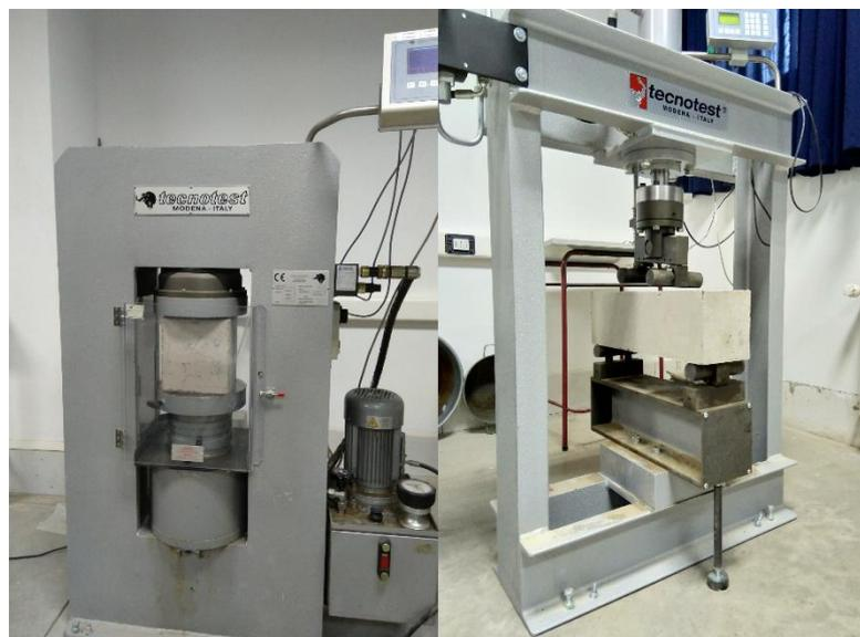
**Figure 3.** Blocks compression and flexural tests.
