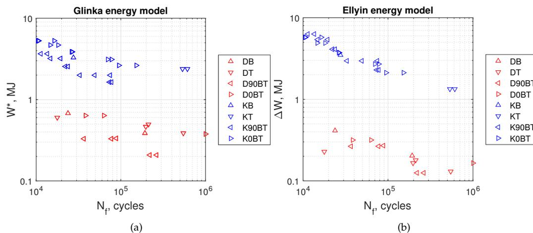
**Figure 15.** (a) Glinka parameter in Equation (9), (b) Ellyin energy parameter in Equation (11). Tests at kinematic load: K90BT, out of phase; K0BT, in phase; KB, bending; KT, torsion. Dynamic loads: D90BT, out of phase; D0BT, in phase; DB, bending; DT, torsion.
