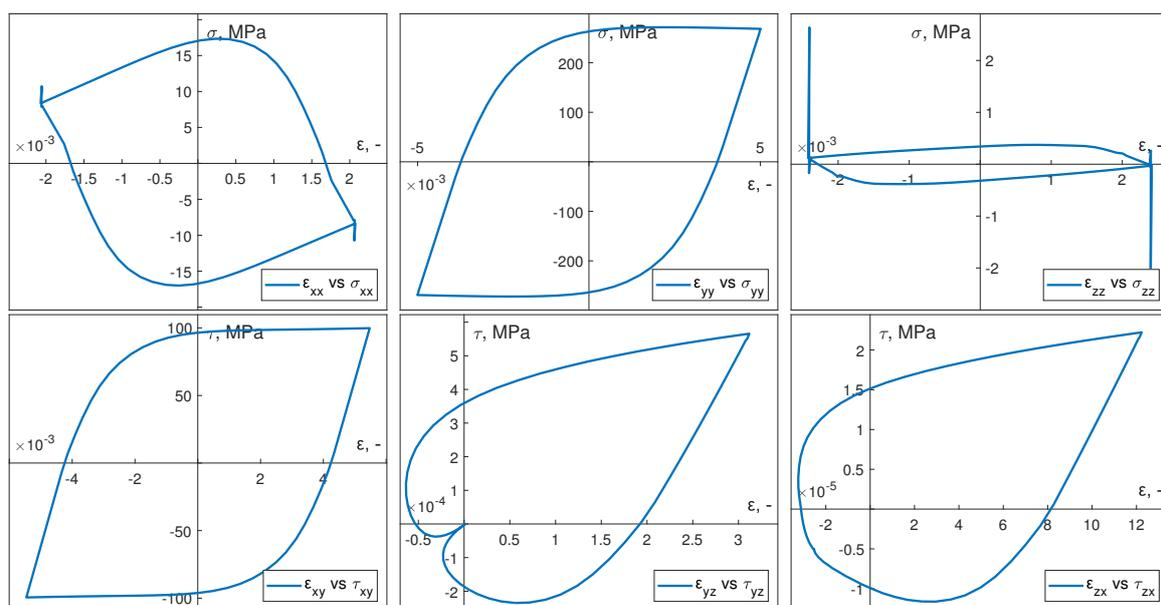
Figure 6. Numerical obtained hysteresis loops for in-phase kinematic load.
