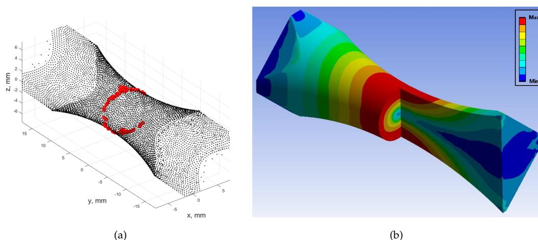
**Figure 19.** (a) Distribution of the most stressed mesh nodes calculated according to the von Mises criterion for in-phase kinematic loading; (b) Area of occurrence of plastic strains FEM calculated for the Chaboche cyclic plasticity model for out-of-phase kinematic loading.
