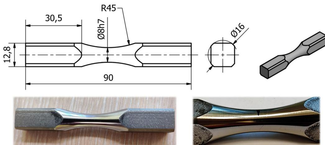
Figure 1. Test specimen. All dimensions are provided in millimeters.
