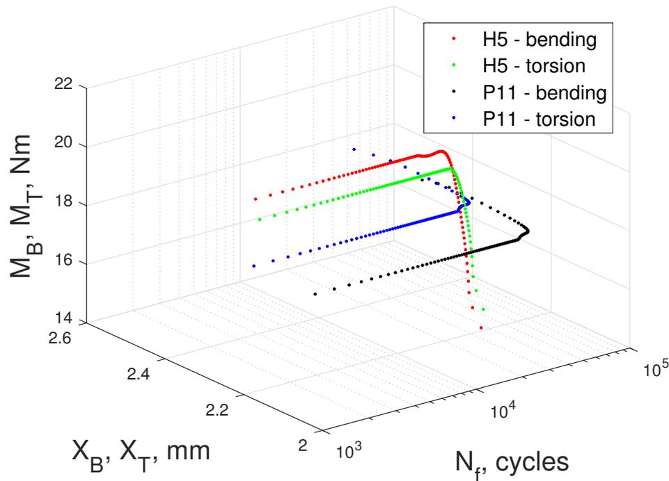
**Figure 16.** Change in recorded values of bending and torsional moments of specimen No. H5 during the entire test period under kinematic load (red and green) and change in the value of the machine lever displacement for dynamic load for specimen no. P11, black and blue.
