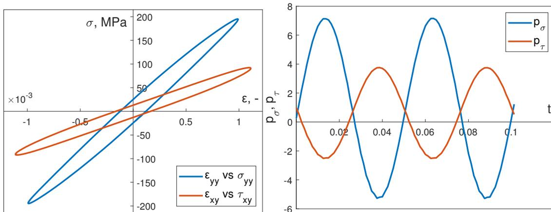
**Figure 12.** Stabilized calculated hysteresis loops for dynamic out-of-phase load and calculated instantaneous power (bending)  $p_\sigma$  and torsion  $p_\tau$ .
