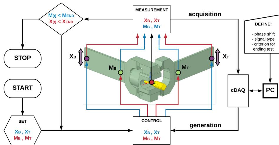
Figure 3. Fatigue machine control and conditioning system.
