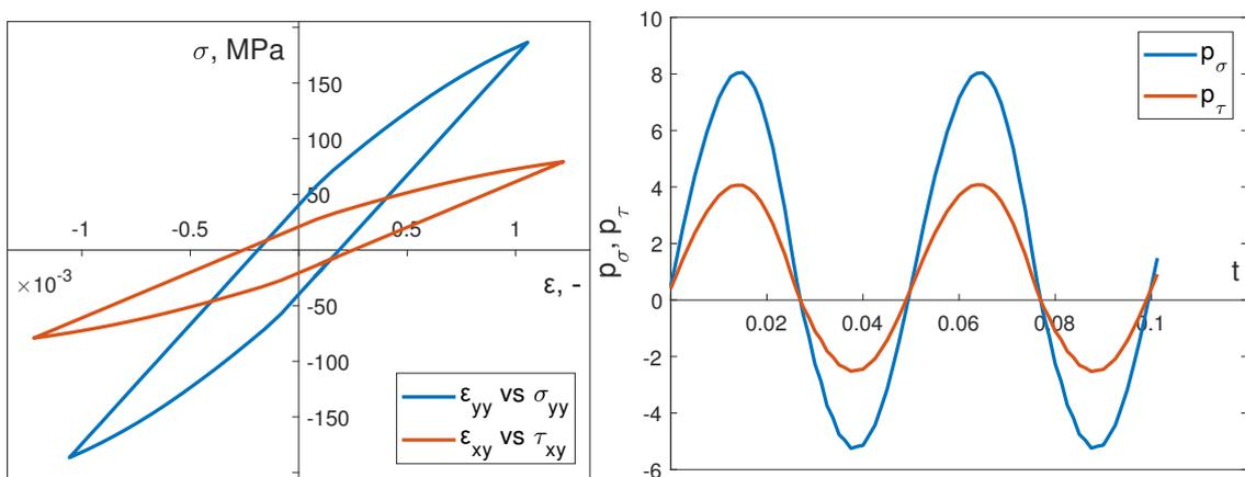
**Figure 11.** Stabilized calculated hysteresis loops for dynamic in-phase load and calculated instantaneous power (bending)  $p_\sigma$  and torsion  $p_\tau$ .
