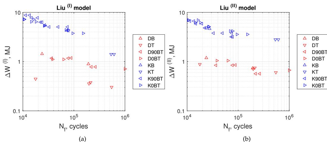
**Figure 14.** (a) Liu <sup>(I)</sup> model Equation (7), (b) Liu <sup>(II)</sup> model Equation (8). Tests at kinematic load: K90BT, out of phase; K0BT, in phase; KB, bending; KT, torsion. Dynamic loads: D90BT, out of phase; D0BT, in phase; DB, bending; DT, torsion.
