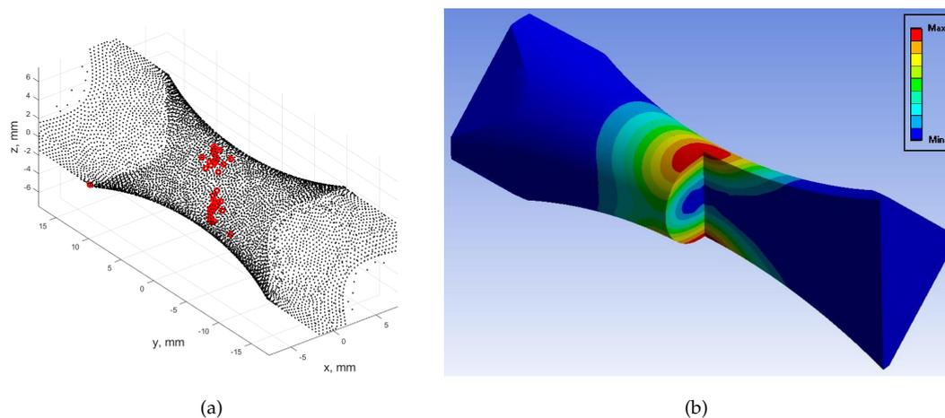
**Figure 18.** (a) Distribution of the most stressed mesh nodes calculated according to the von Mises criterion for in-phase kinematic loading; (b) Area of occurrence of plastic strains finite element method (FEM) calculated for the Chaboche cyclic plasticity model for in-phase kinematic loading.
