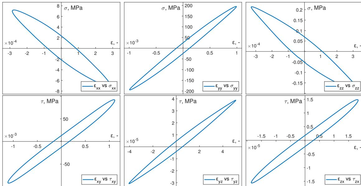
**Figure 7.** Numerically calculated hysteresis loops for out-of-phase dynamic load.
