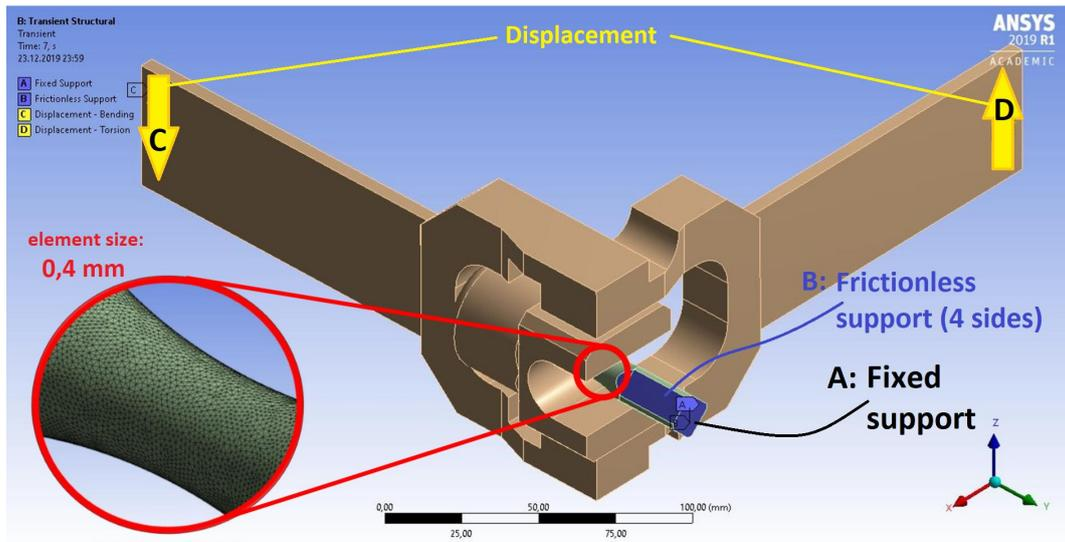
Figure 5. Numerical model of clamping/loading system of the fatigue machine.
