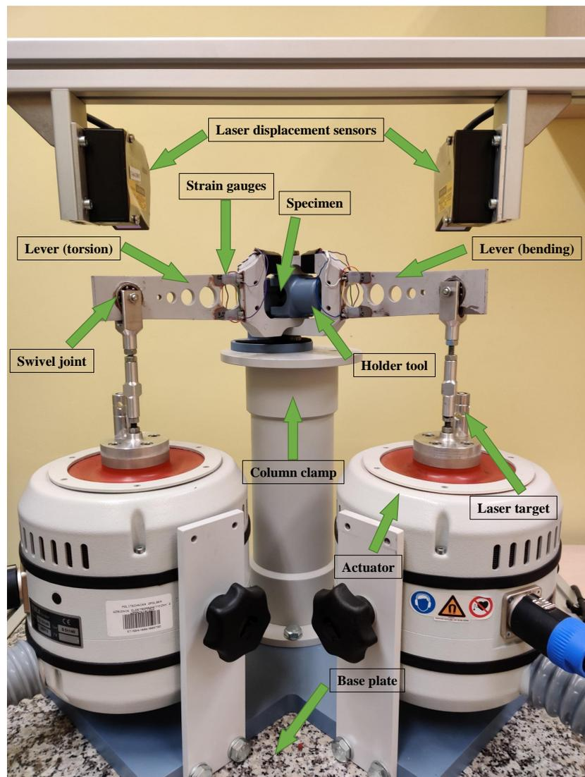
**Figure 2.** Fatigue testing machine.
