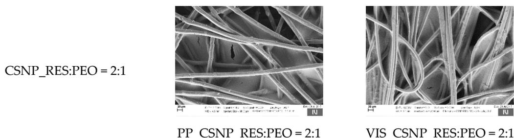
**Figure 2.** Scanning electron microscopy (SEM) images of liquid formulation samples CSNP:PEO = 2:1, CAT:PEO = 1:2, RES:PEO = 1:2, CSNP\_CAT:PEO = 2:1 and CSNP\_RES:PEO = 2:1, electrospun onto the polypropylene substrate material (left) and on viscose substrate (right).
