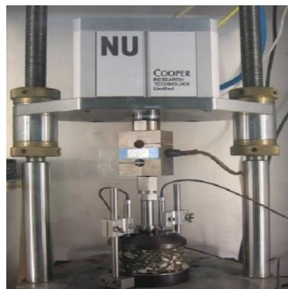
**Figure 4.** Dynamic creep test of asphalt mixture.
