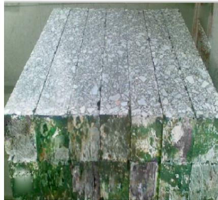
Figure 7. Beam samples for four point bending fatigue test.
