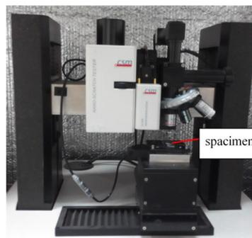
Figure 1. CSM Tribo-Indenter and the specimen.
