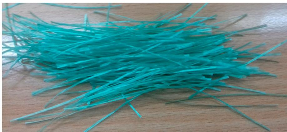
**Figure 2.** Photograph of the obtained copper alginate fibers.
