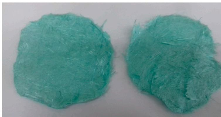
**Figure 3.** Photograph of nonwovens made of copper alginate fibers.
