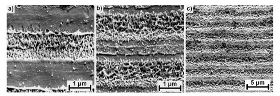
**Figure 7.** High magnification images of a tungsten surface irradiated with 1 mJ (0.81 J/cm<sup>2</sup>) and a single pulse (**a**), 5 pulses (**b**), and 10 pulses (**c**). All images are captured with the sample tilted 55°.
