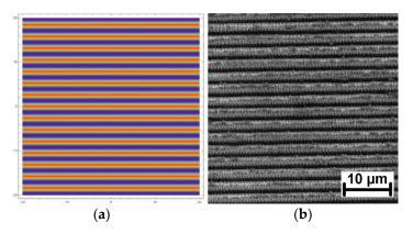
**Figure 1.** (a) Calculated pattern for two beam interference with a periodicity of 2.64  $\mu$ m; (b) SEM image of the pattern fabricated on stainless steel with the same periodicity.
