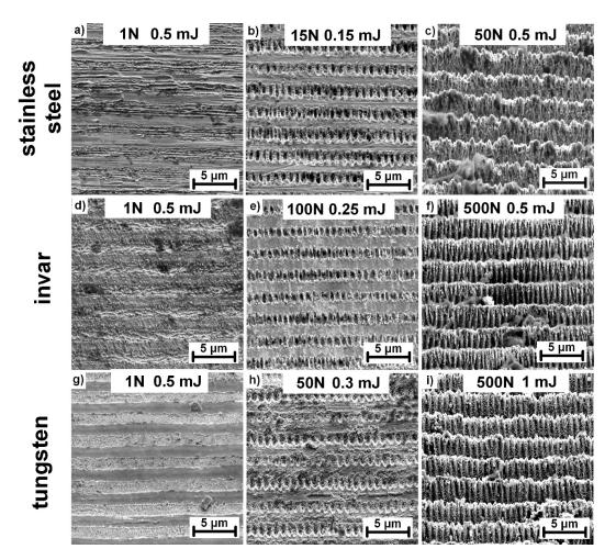
**Figure 6.** Different surface morphologies achieved by variations in the pulse energy and number of pulses (N) on invar (**a**–**c**), stainless steel (**d**–**f**), and tungsten (**g**–**i**). All images were captured with the sample tilted 55°.
