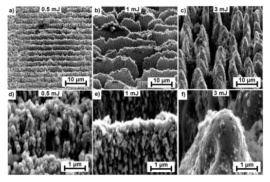
**Figure 4.** Structure evolution on a stainless-steel surface with increased pulse energy and 1000 consecutive laser pulses. Detail images with higher magnification are shown in the second row with the corresponding pulse energy. All images were captured with the sample tilted 55°.
