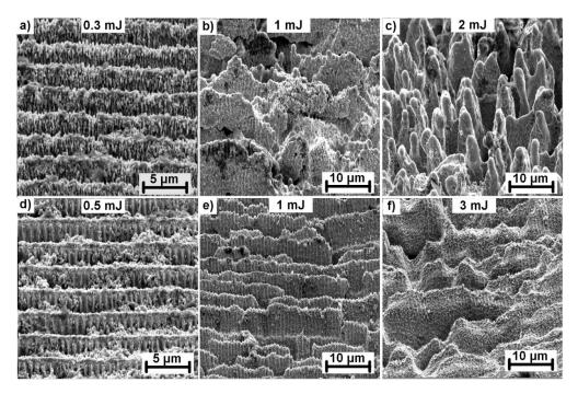
**Figure 5.** Structure evolution in Invar (**a**–**c**) and tungsten (**d**–**f**) with increasing pulse energy. The surface was irradiated with 1000 consecutive laser pulses. All images were captured with the sample tilted 55°.
