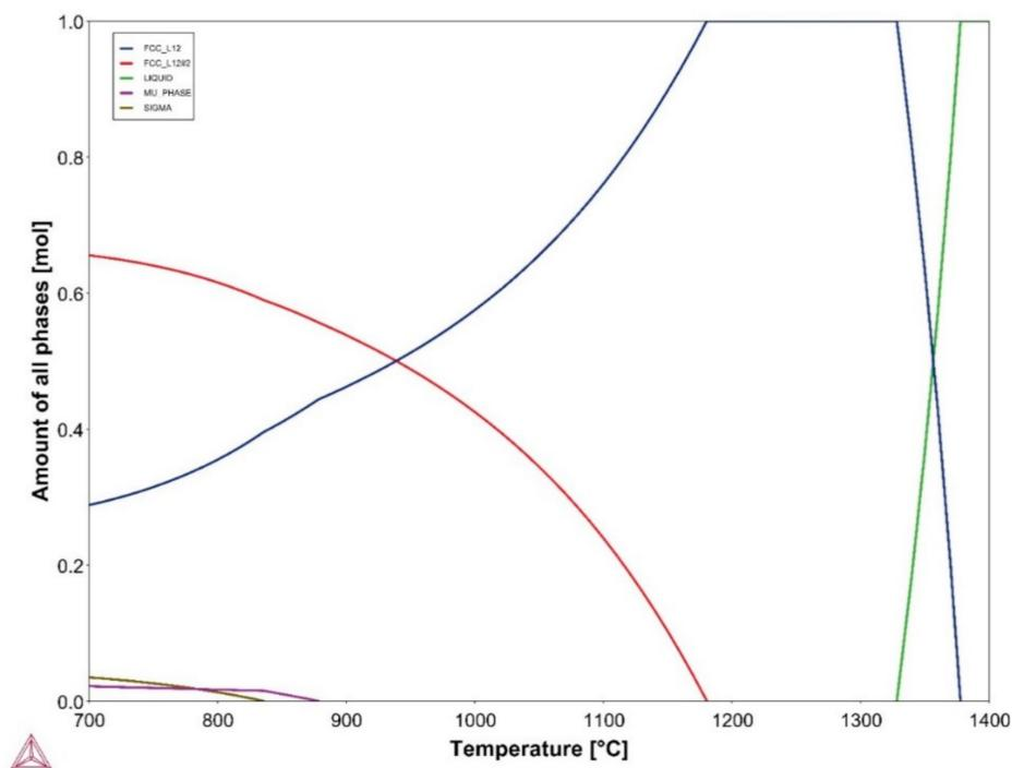
**Figure A1.** The thermodynamic equilibrium step diagram of MAD542 using the TCNI10 database in the Thermo-Calc software.
