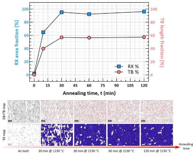
**Figure A4.** The twin boundary (TB) and recrystallization (RX) fraction evolution as a function of annealing time at 1230 °C, indicating a combination of rapid RX and TB formation processes. The EBSD scans cover an area of 870 μm × 1266 μm with a 2-μm step size. In the GB + TB maps, the grain boundaries (GB) are plotted in black lines, while TBs are plotted in red lines. In the RX maps, RXed grains are colored in blue. All the scale bars are 125 μm.
