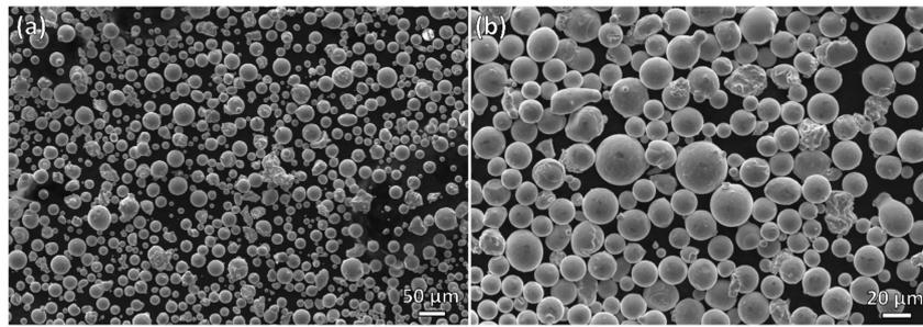
**Figure A2.** Secondary electron SEM micrographs of the virgin powders of the MAD542 superalloy for laser powder bed fusion. (a) at low magnification with an overall view and (b) at high magnification with a detailed view.
