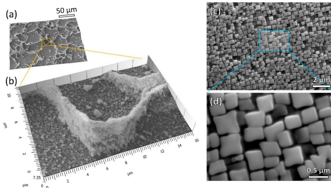
**Figure 4.** The  $\gamma'$  precipitate morphology of MAD542 superalloy after post-processing heat treatment. (a) Stereo-image from SEM-secondary electron (SE) micrographs on a deep etched sample, showing a high amount of  $\gamma'$  precipitate decorating the grain boundary region with an enlarged view in (b); (c) SEM-SE imaging of high density of  $\gamma'$  precipitates observed in the grain interior region; (d) the enlarged view of cuboidal  $\gamma'$  morphology.
