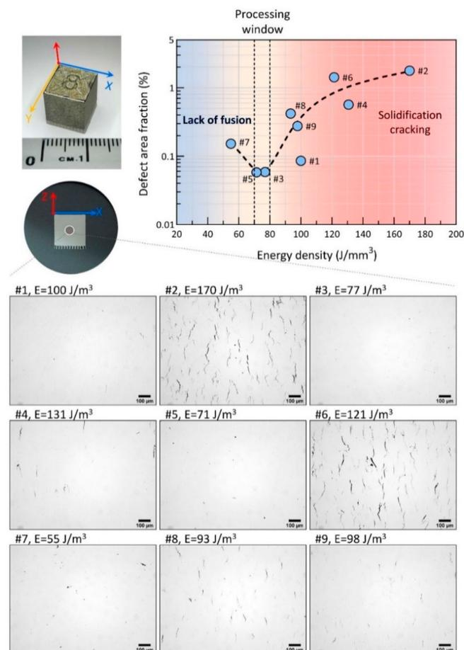
**Figure 1.** Laser powder bed fusion (LPBF) processing window investigation of MAD542 superalloy on 10 mm × 10 mm × 10 mm cubes. With lower energy density input, the major defects are dominated by lack of fusion, while higher energy density inputs result in micro-cracks. The crack-free part is provided by #3 printing parameters, which has a suitable energy density input for MAD542.
